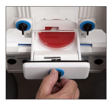
Introduce individual samples without compromising internal atmospheric conditions
