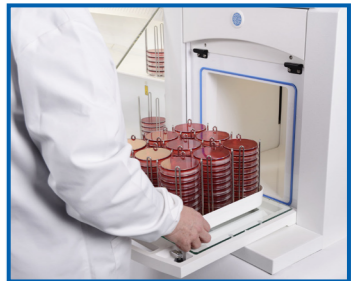
The airlock can transfer items of equipment or up to 90 x 90mm Petri dishes in only 5 minutes.
