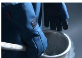
**5** Cryo gloves protect your hands and prevent frost bites when handling samples which are stored at down to -160 °C.
