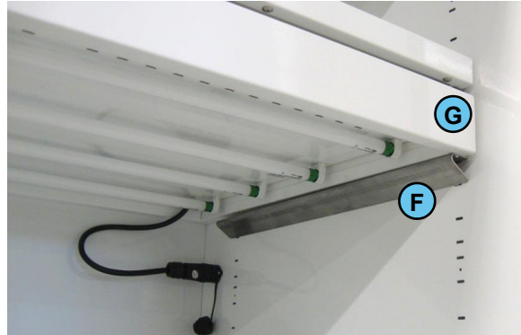
Figure 2-6 TC Lamp Canopy Supports Detail
