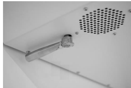
Figure 5-2 Damper Adjustment Lever
