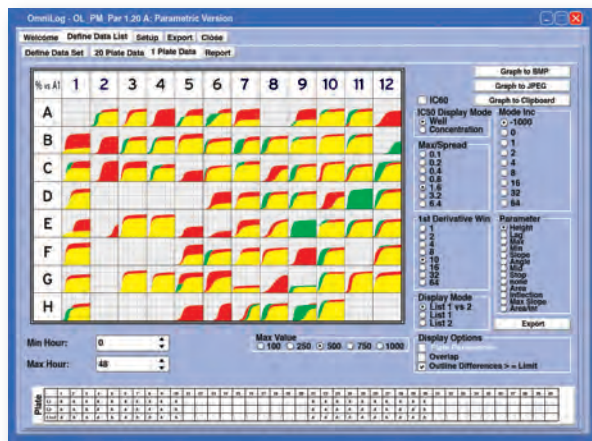
Phenotype MicroArray Single Panel Comparison Display showing Cellular Responses for 96 Kinetic Assays
