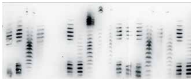
IEF results of EPO standards using SERVA EPO Doping gel kit. With courtesy of Institute of Doping Analysis and Sports Biochemistry, Kreischa. Accredited WADA laboratory.
