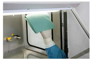
**Drops of detergent and contaminants** can fall outside the cabinet toward floor or operator!
