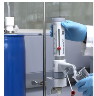
Remote Dispensing System for Drum Dispensing
