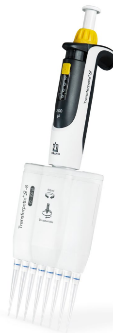
Individually exchangeable shafts on the Transferpette® S-8 and -12
