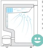
BioCompact 210 Refrigerator with a finned tube evaporator enables forced air distribution inside the storage chamber. Thereby evenly distributing cold air throughout, enhancing temperature stability and uniformity. Using a finned tube evaporator and placing it away from the storage chamber eliminates cold walls. A fan forces cooled air around the cabinet to ensure even distribution.
