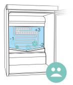
Conventional refrigerator with evaporator in the storage space, evaporating refrigerant lowers temperature by absorbing heat and transferring it outside the cabinet.
