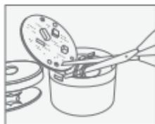
4. Cut the wires from PCB.
