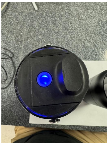
Figure 2. Testing of the Larq device whereby the unit was turned on with a double press of the button, resulting in a dark blue pulse every 1 second. The unit was maintained in a upright position on the countertop and moved in a circular motion.
