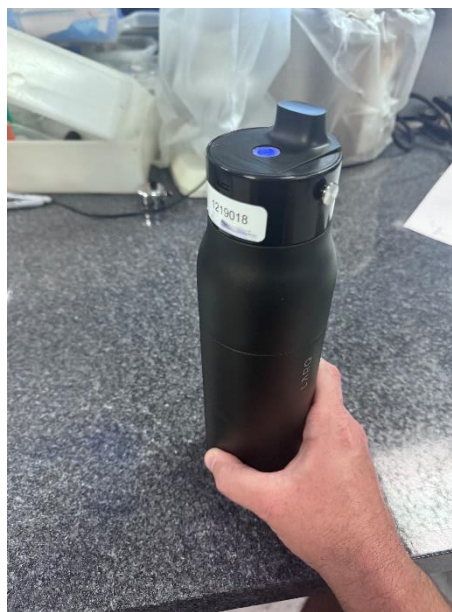
Figure 2. Testing of the Larq device whereby the unit was turned on with a double press of the button, resulting in a dark blue pulse every 1 second. The unit was maintained in a upright position on the countertop and moved in a circular motion.
