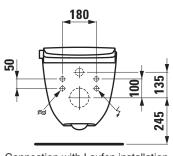
Connection with Laufen installation system LIS CW2
