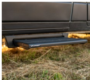
Lightweight, durable plastic, steel, and aluminum construction with anti-slip surface for safe stepping
