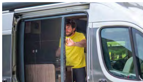
Clutched sliding system allows the screen to be opened to any position
