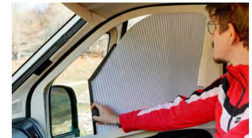
PVC and aluminum handle for manual operation
