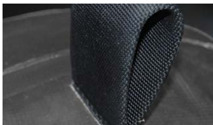
2" tubular nylon webbing exceeds 4,500 lbs. tensile strength
