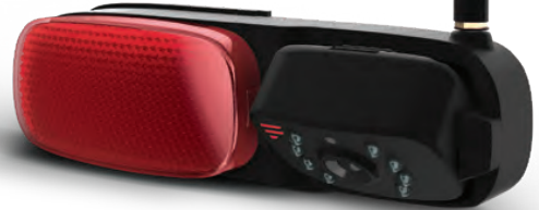
Rear Camera with LED Marker Light
