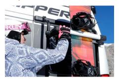
Ergonomic release button for comfortable unloading
