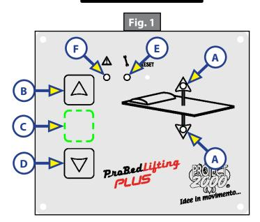
2. A hidden (NULL) button (Fig. 1C) is located between the UP and DOWN buttons to initiate the stop position program and to set the stop positions. To initiate the stop position program use steps A-C.
