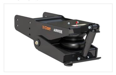
This pin box is uniquely constructed with a built-in shock that protects the air bag from destruction by recoiling the pin box, along with a scissor-like motion that allows it to compress, offsetting bounce and providing cushion
