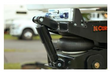
This pin box contains an internal air bag that moves in a scissor-like motion to absorb vibrations, a rubberized compound to soften jarring movement, and an oil shock absorber to handle rebound action, dampen kickback and control chucking
