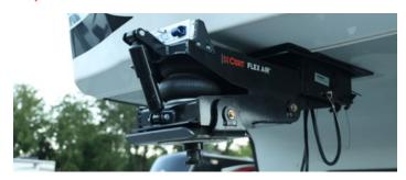
The Flex Air 5th wheel pin box combines our time-tested Air Ride technology with our Rota-Flex pivoting head to significantly reduce fore to aft movement and vertical tug-of-war between a 5th wheel RV and tow vehicle
