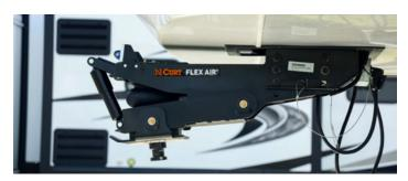
Constructed with steel and a black powder coat finish that protects against rust, this pin box is extremely durable to ensure peaceful towing day after day
