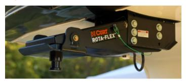
The Rota-Flex features a pivoting head that moves and controls back and forth movement of the king pin within the hitch which significantly reduces chucking and provides a smoother ride
