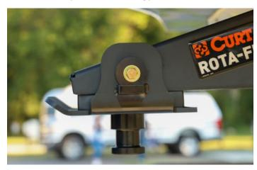
To minimize strain and reduce wear and tear on the trailer, the Rota-Flex contains a robust rubber compound in its head that absorbs the road shock, bumps, and vibrations experienced on rugged terrain
