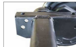
Square pattern torsion axle
