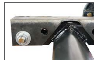
Diamond pattern torsion axle
