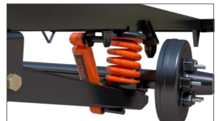
Trailing arm style suspension with coil springs and shock absorbers
