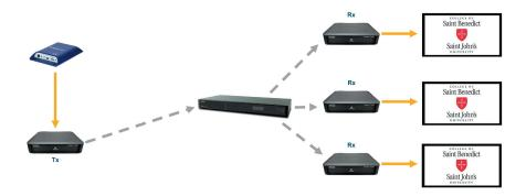
Add a Tx/Rx in transmit mode and input your media source. Next, set any number of Tx/Rx units to receive, and from the web interface, select the source you would like them to receive. Connect the receiving units to a display or a projector and your content distribution setup is complete.
