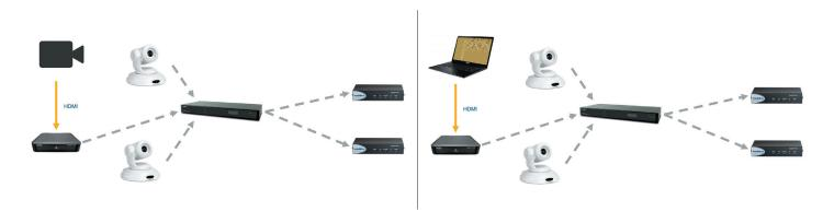
In a conference room, you can add a third-party HDMI camera or an HDMI content source to your existing EasyIP system. Simply add an EasyIP Tx/Rx in transmit mode to convert the HDMI signal to EasyIP.
