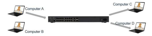
Multicast (on an unmanaged or unconfigured switch)
