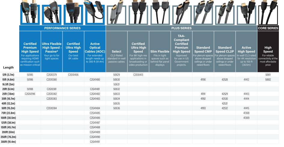
\*Passive HDMI cables have limited maximum lengths, while Active HDMI cables feature an on-board processor which boosts the signal. making them the clear choice for installations of longer distances.
