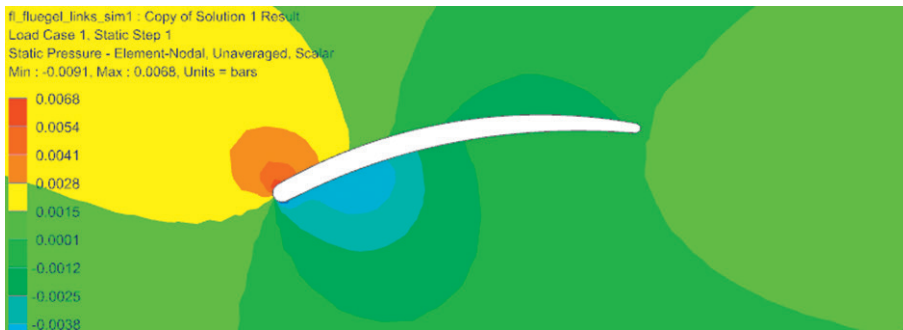
Figure 30 The static pressure distribution is plausible for an airfoil.
