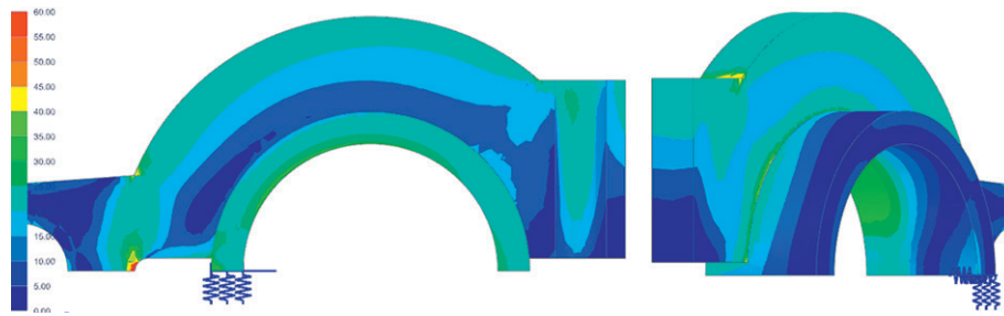
Figure 23 The von Mises stresses
