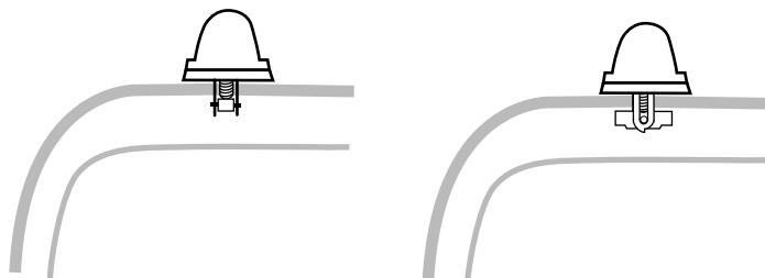
**17** Screw bolt into fastener. Do not fully tighten.
