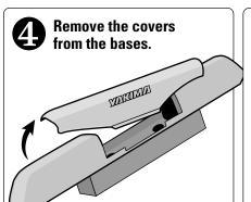
When the racks are not installed, use the covers to keep the bases free of debris.
