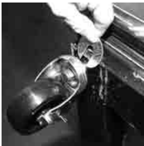
For leveling, insert the shim between the caster and frame rail.
