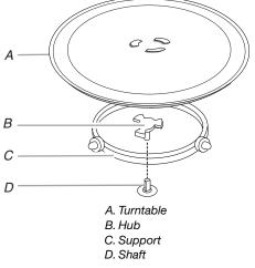
The turntable can rotate in either direction to help cook food more evenly. For best cooking results, do not operate the microwave oven without having the turntable in place. See "Assistance or Service" to reorder any of the parts.
