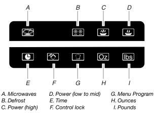
The icons light up in the display while their specific functions are being programmed. While the set function is operating, the icons flash until the program is over. The control lock icon remains lit – not flashing – while the control is locked.
