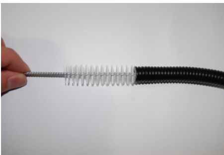
Fig. 66: Clean pump hoses
