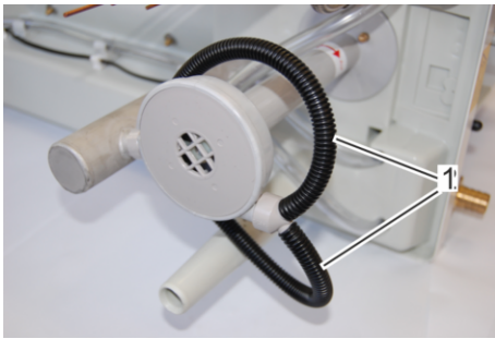
Fig. 50: Attach pump hoses
