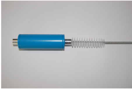
Fig. 69: Cleaning the lime transforming cartridge
