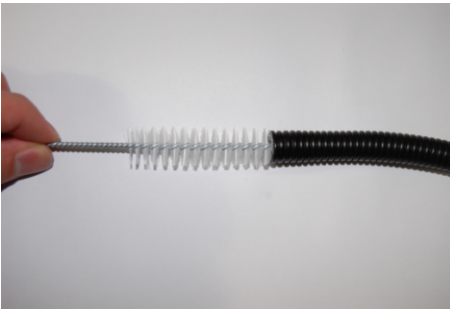
Fig. 39: Clean pump hoses
