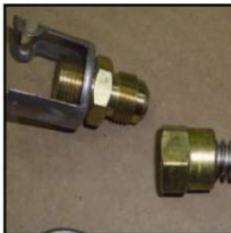
Step 4. Remove brass orifice from flex line.
