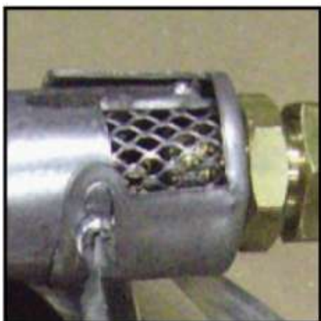
Step 3. Remove shutter screw and slide off.
