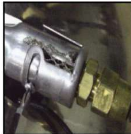
Step 5. Follow the above steps 3 and 4 in reverse order with new natural gas orifice. Set shutter opening to closed position. No screen showing for Natural Gas.
