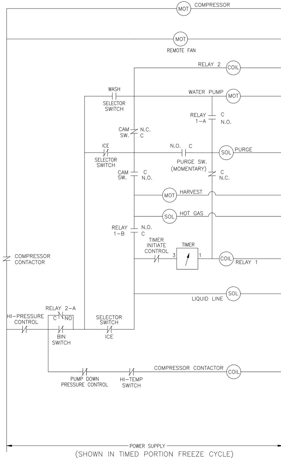
ICE1405/6A3/W3, ICE1806W3 and ICE2106W3 Wiring Diagram
