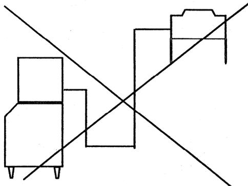
**DO NOT** Install the condenser lower than 6' (1.83 meters) below the quick connect fittings at rear of machine.
