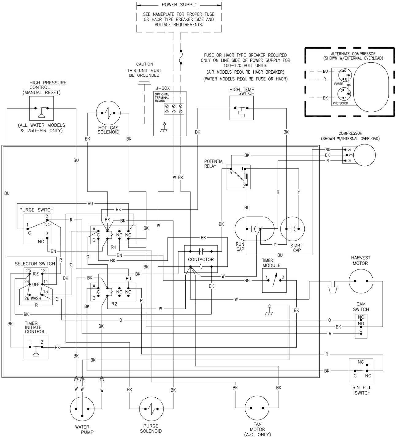
ICE0500 Air and Water Wiring Schematic
