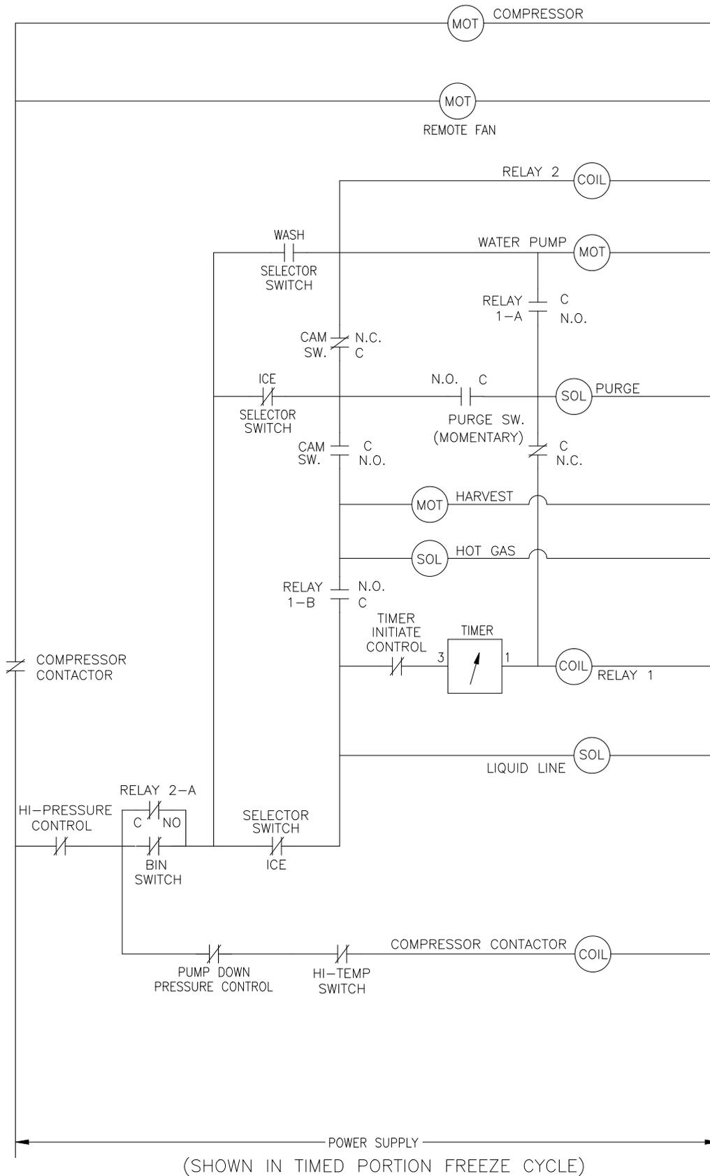
ICE0606 Air3 and Water3, ICE0605 Air3 and Water3 Wiring Diagram
