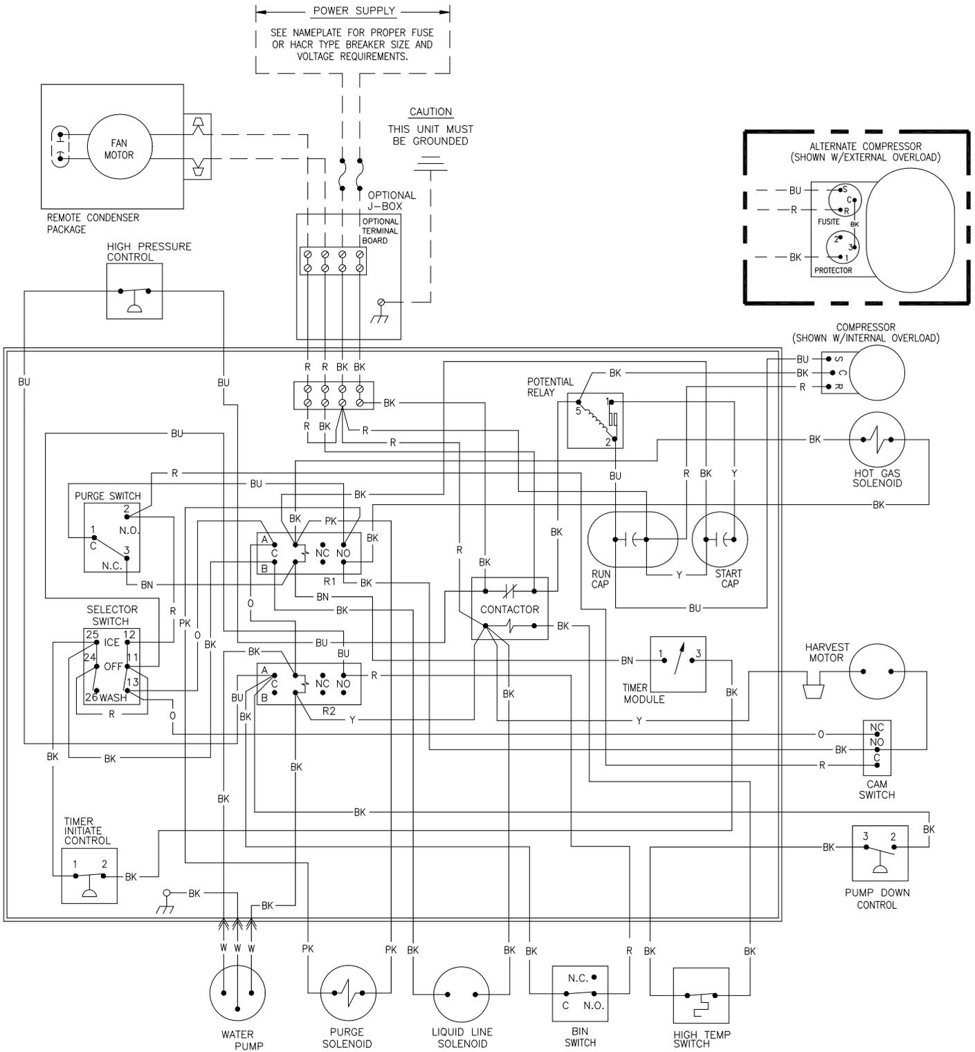
ICE0500 Remote Wiring Schematic (R3)
