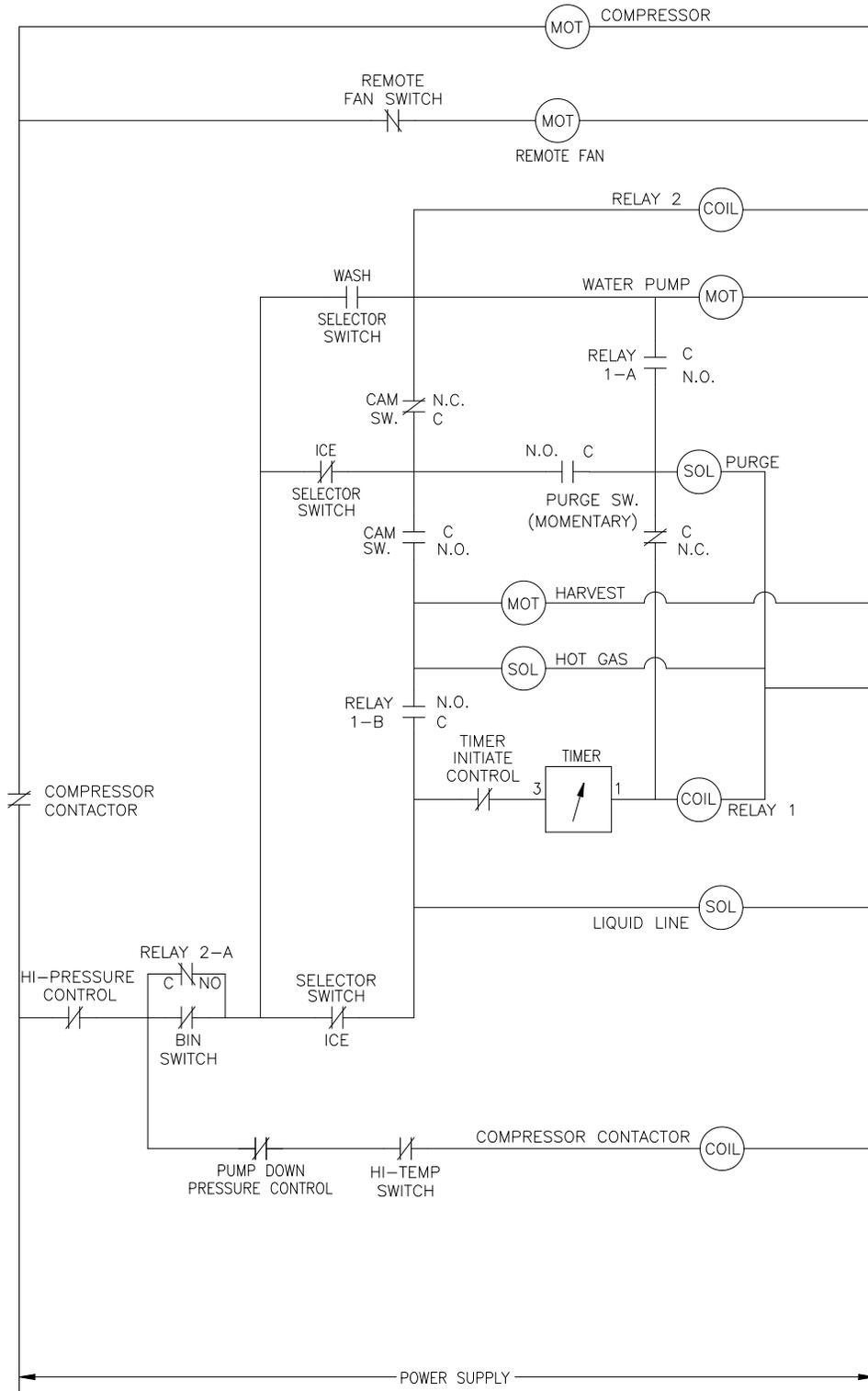
ICE0605/0606/0806/1006 Remote Wiring Diagram (R3)
