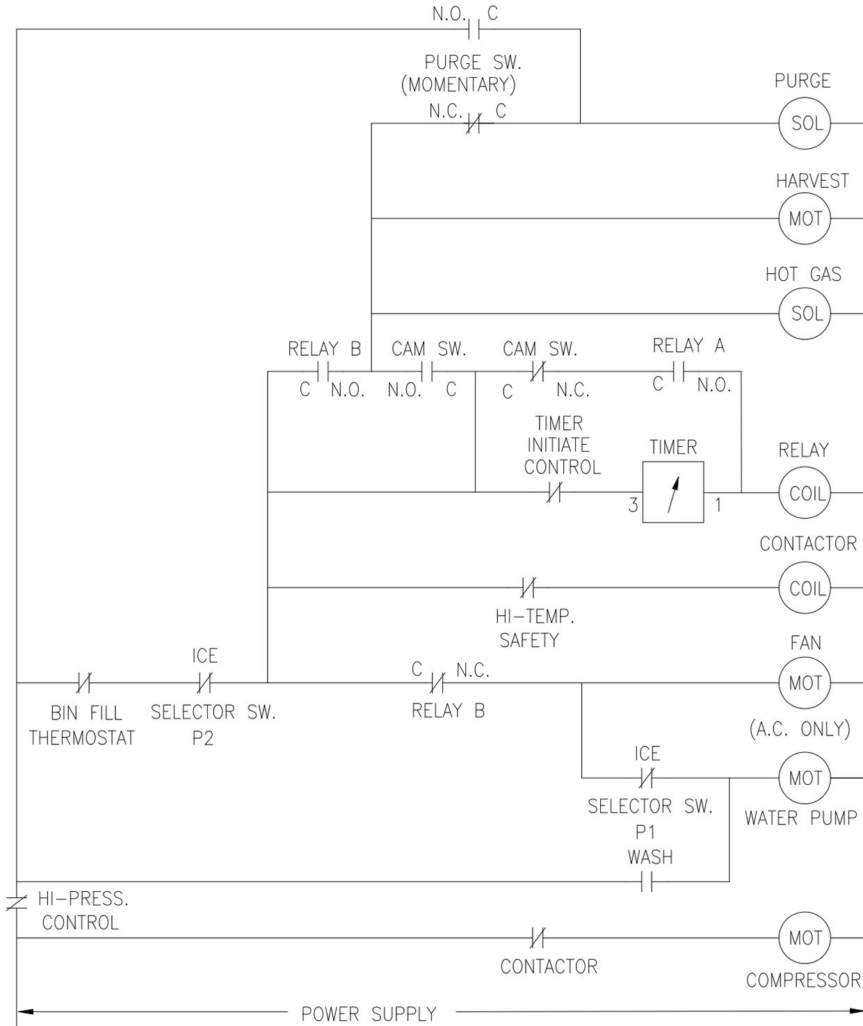
CONTROLS SHOWN DURING TIMED PORTION OF FREEZE CYCLE 9072088-01 REV A
