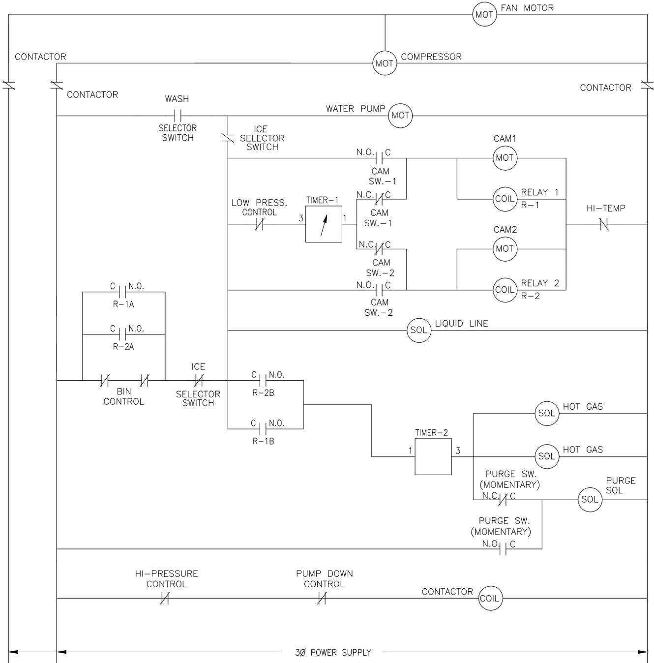
ICE1606 Remote Wiring Schematic
