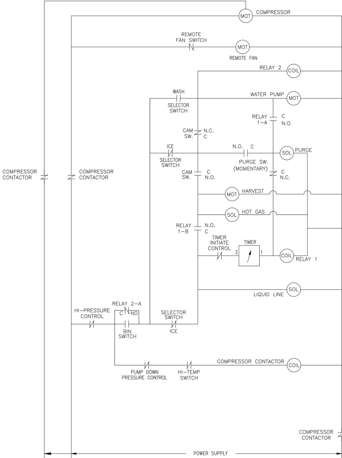
ICE0250 Air4 and Water4, ICE0400 Air3 and Water3 Wiring Diagram
