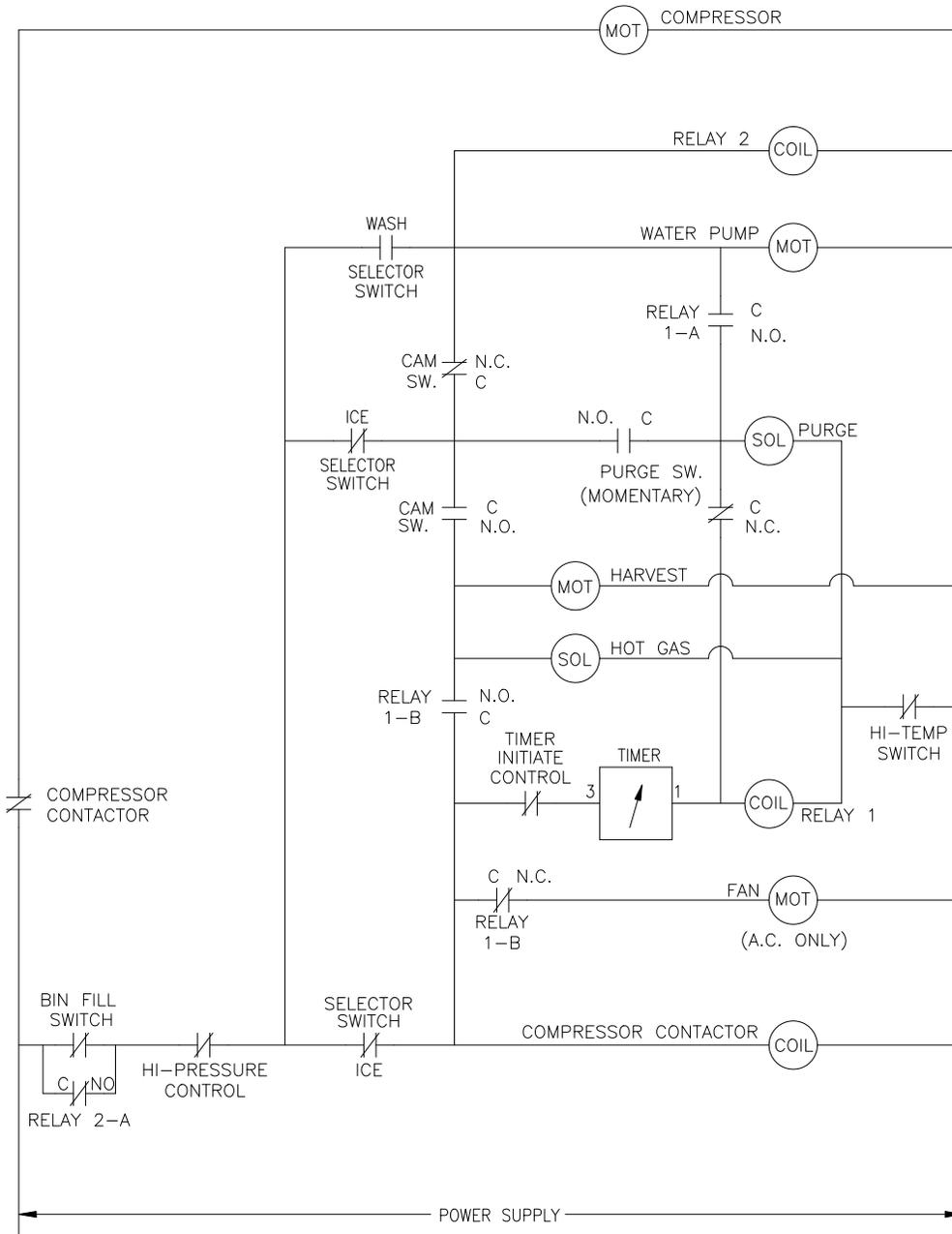
ICE0400 Air and Water Wiring Diagram
