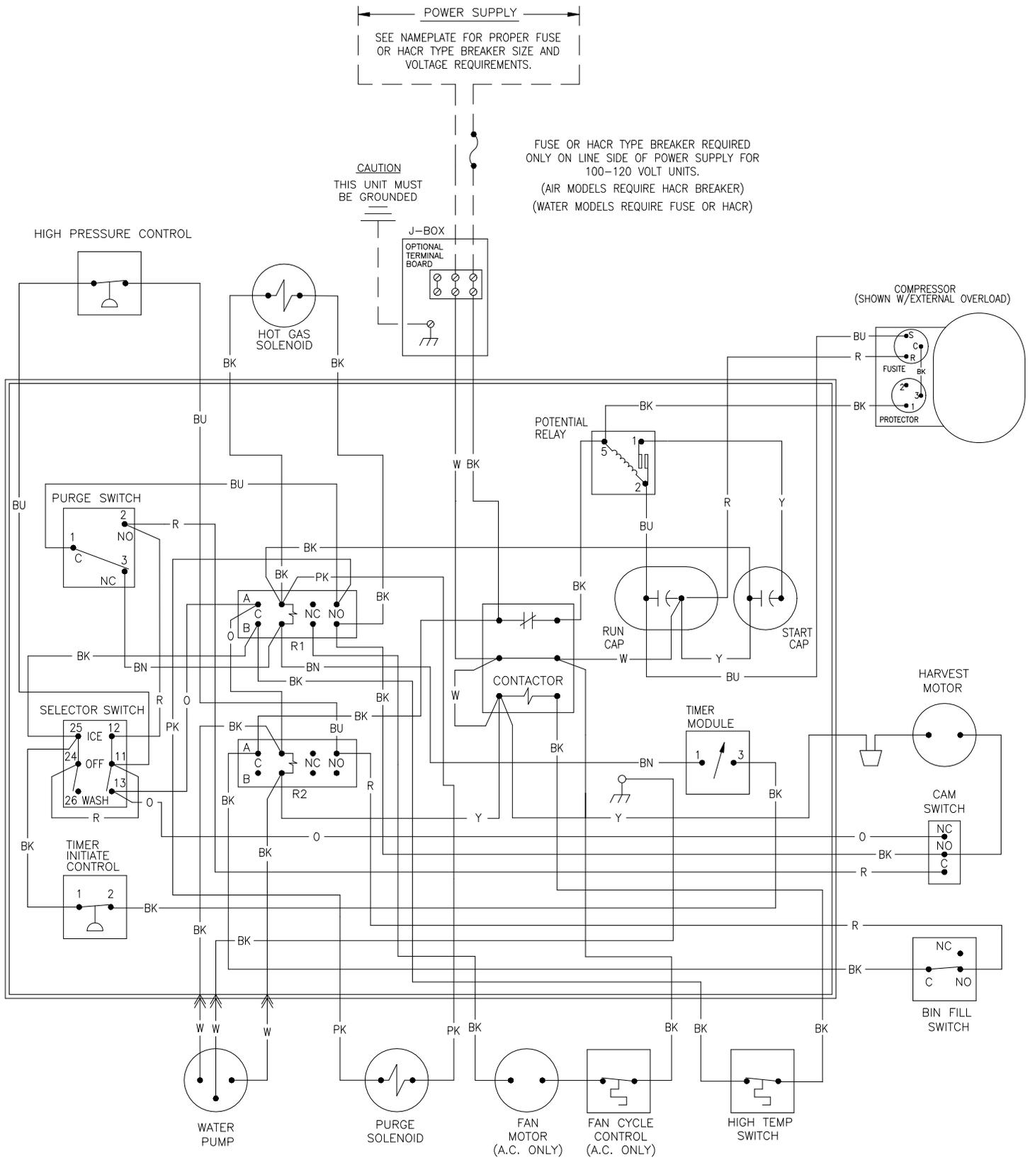
ICE0500 Air3 and Water3 Wiring Schematic
