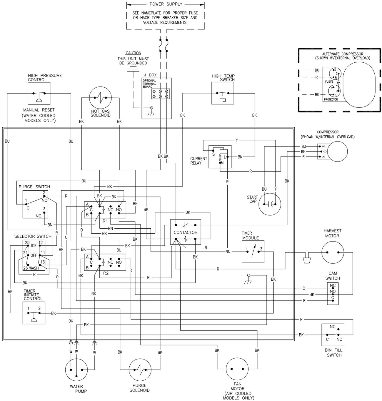
ICE0405/0406 Air and Water Wiring Schematic
