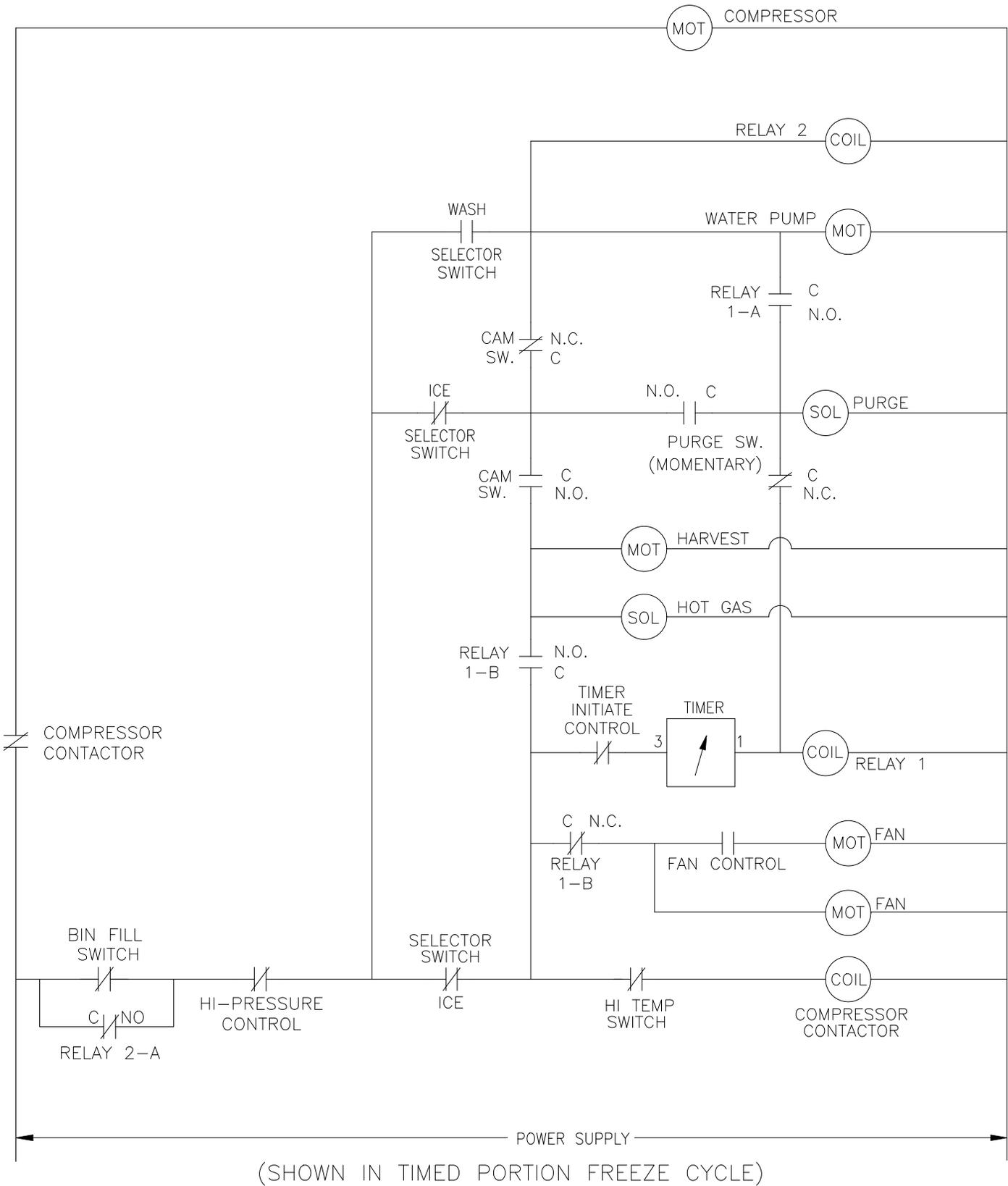
ICE0406/405 Air3 and Water3, ICE0305 Air3 and Water3 Wiring Diagram
