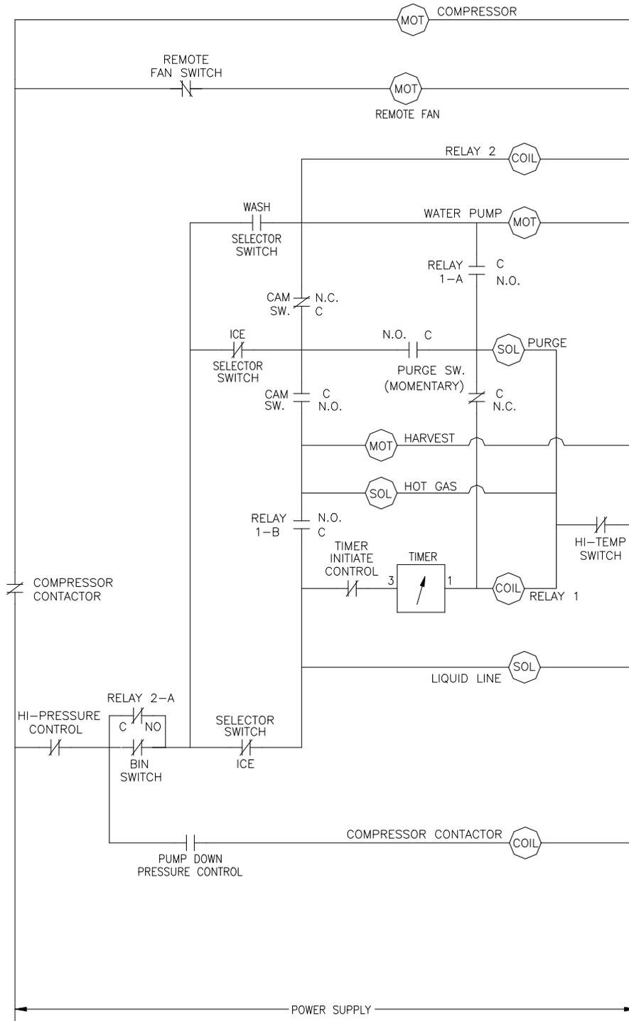
ICE0605/0606/0805/0806/1005/1006 Air and Water Wiring Diagram
