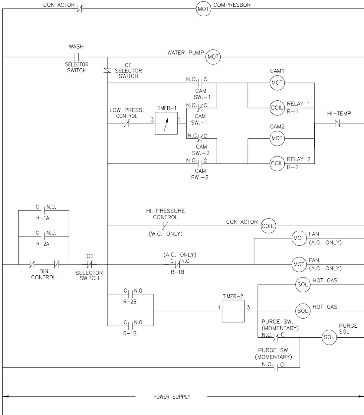
ICE1407/1807/2107 Air and Water Wiring Diagram
