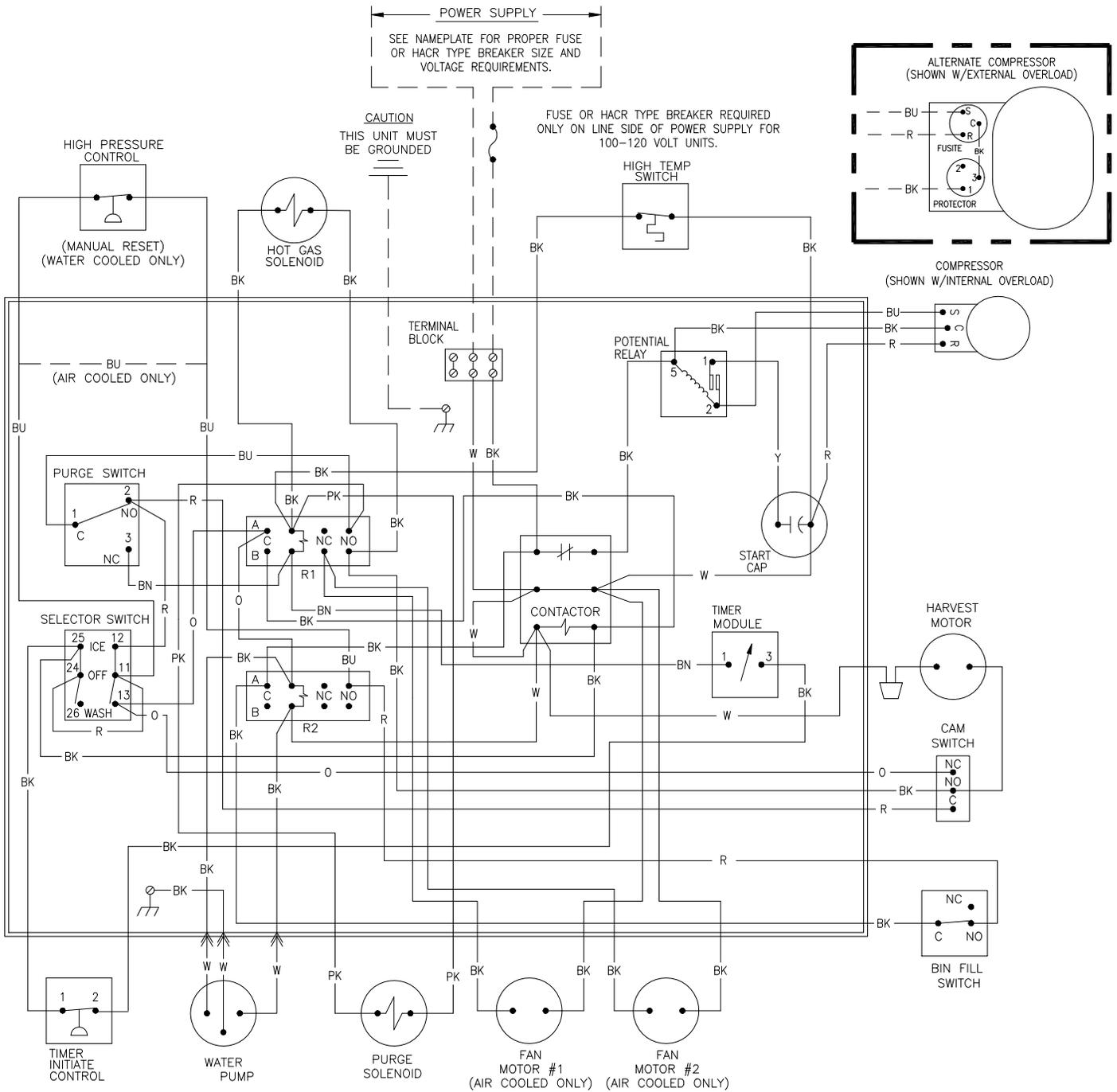
ICE0520 Air and Water Wiring Schematic
