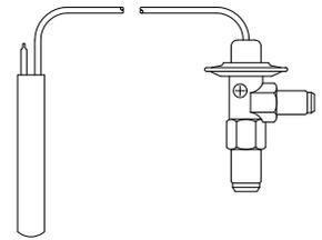
The flow of refrigerant into the evaporator is controlled by the temperature at the outlet of the evaporator. The expansion valve bulb, mounted to the top of the suction line, senses the evaporator outlet temperature causing the expansion valve to open or close. As ice forms on the evaporator, the temperature drops and the flow of refrigerant into the evaporator decreases, resulting in a drop in suction pressure.
