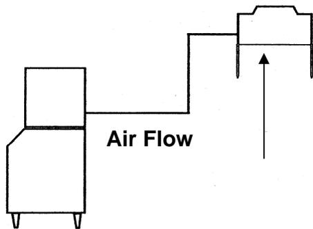
When installing condenser below the ice machine
