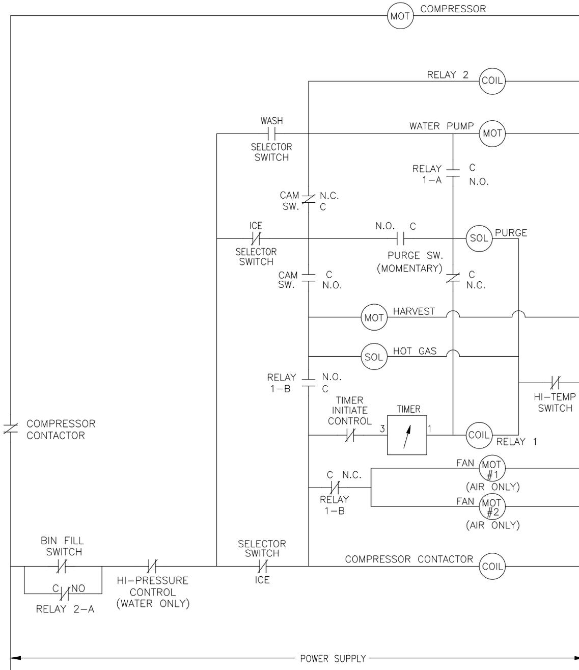
ICE0325/0525 Air and Water Wiring Diagram
