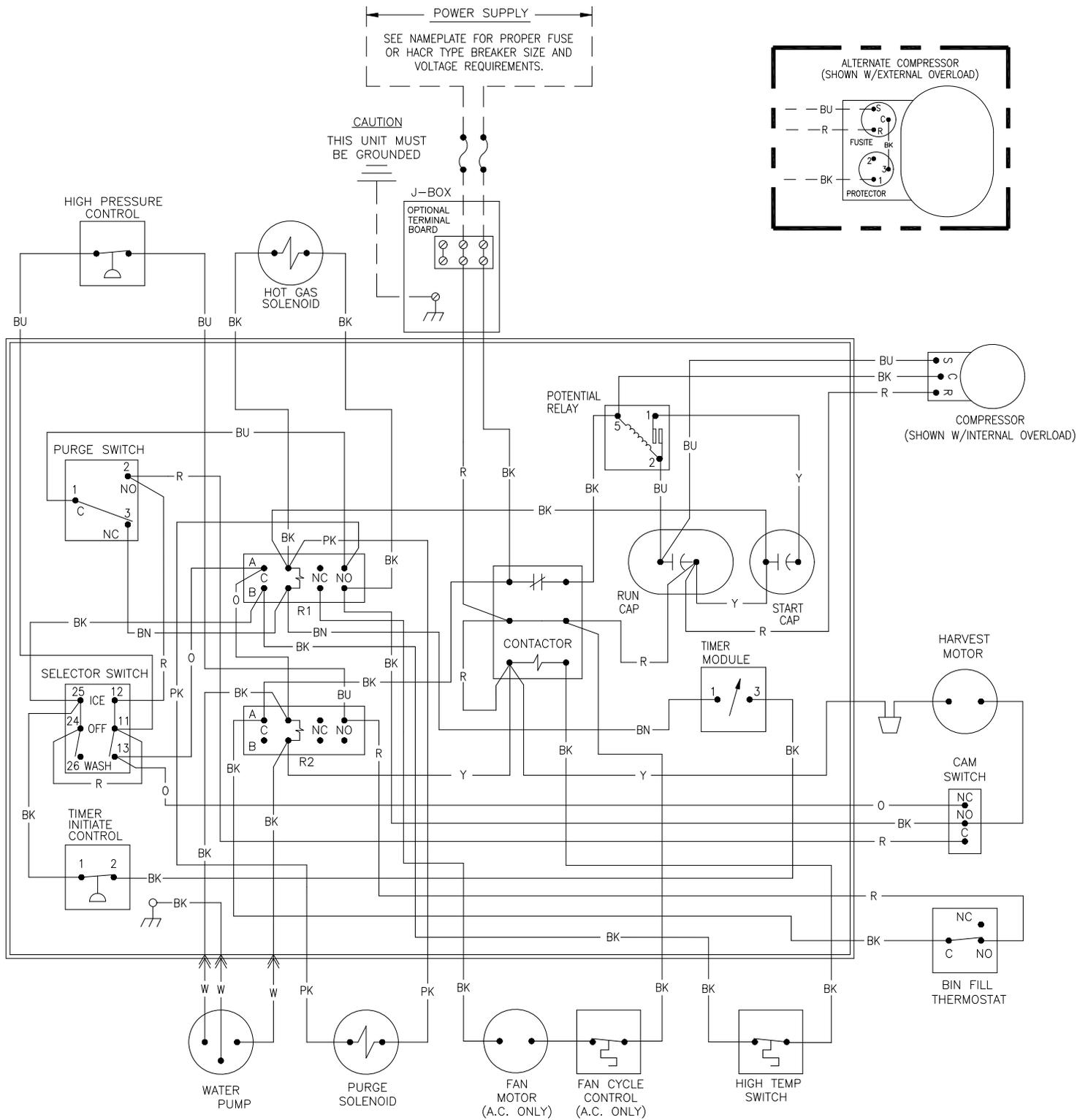
ICE0406/405 Air3 and Water3, ICE0305 Air3 and Water3 Wiring Schematic
