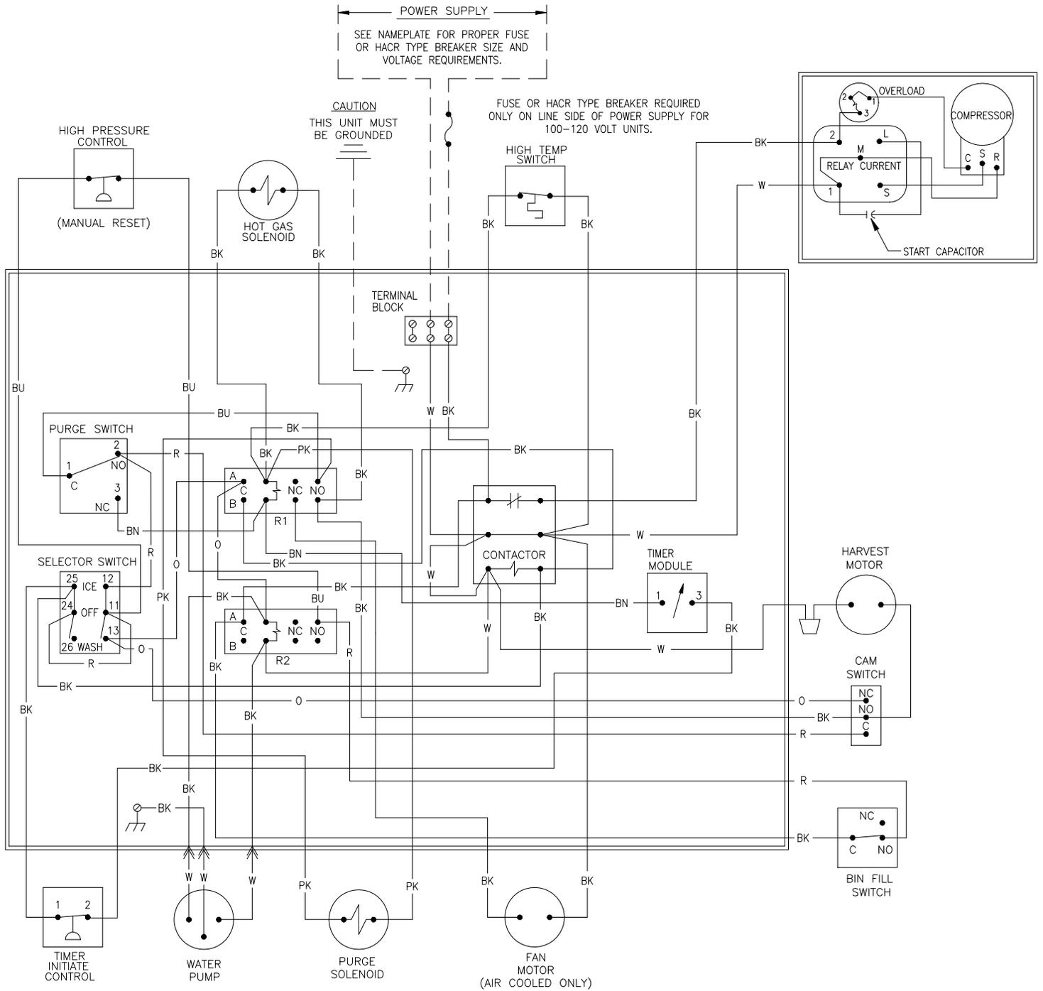
ICE0320 Air and Water Wiring Schematic
