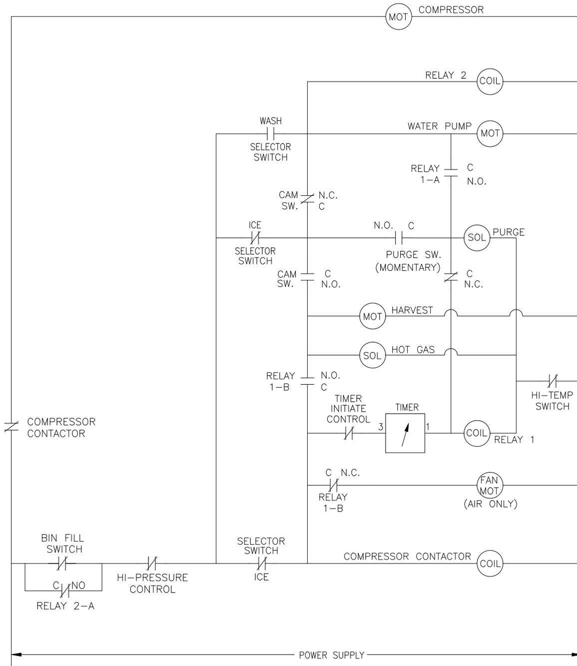
ICE0520 Air and Water Wiring Diagram
