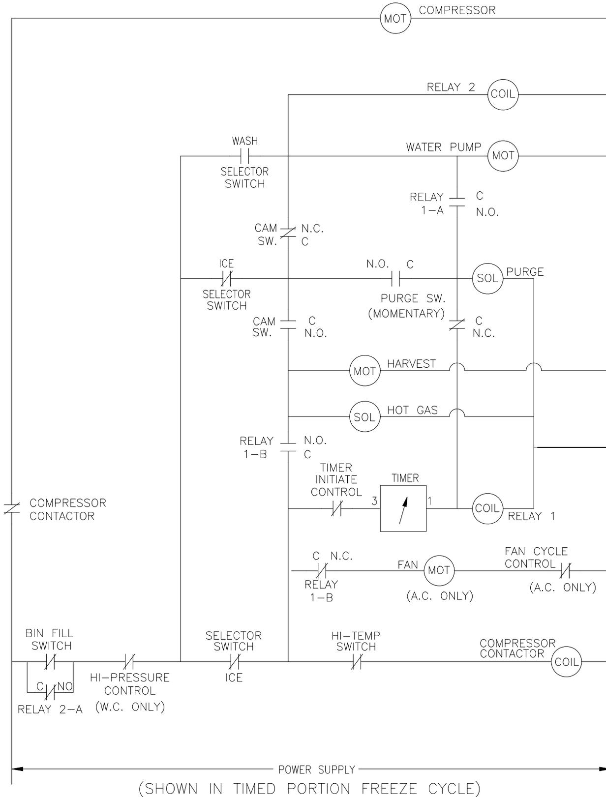
ICE0606 Remote4&5 and ICE0605 Remote4&5 Wiring Schematic
