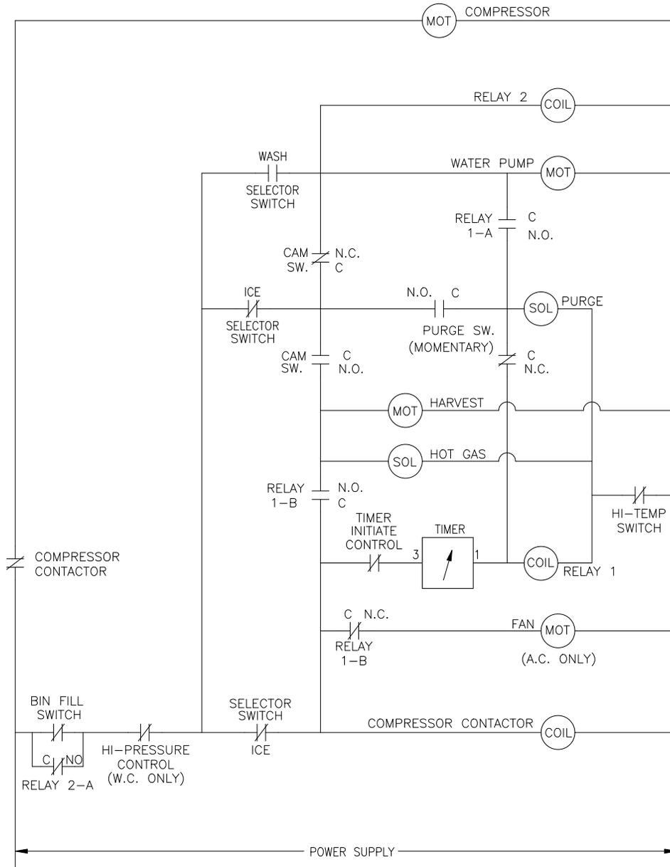
ICE0405/0406 Air and Water Wiring Diagram
