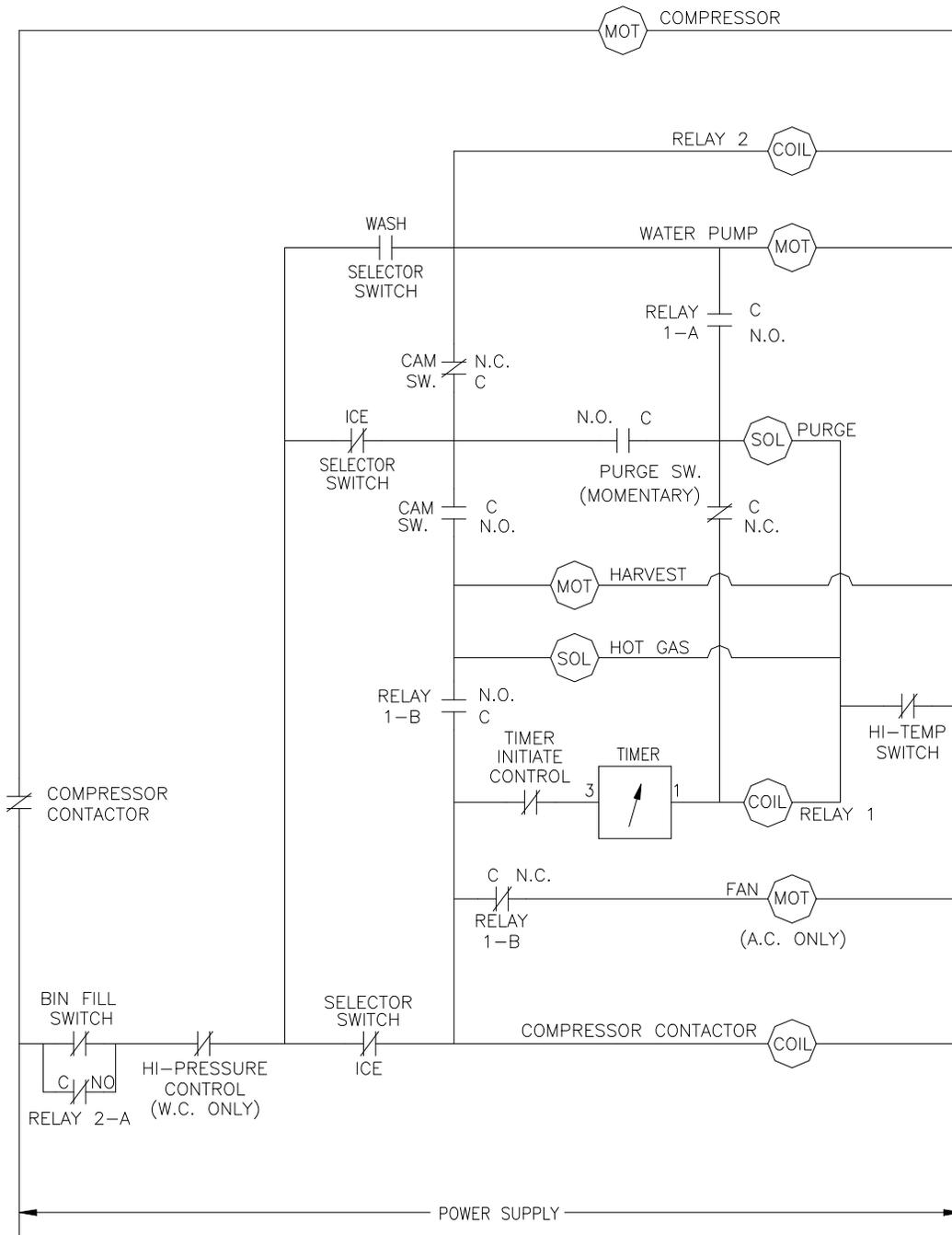
ICE0605/0606/0805/0806/1005/1006 Remote Wiring Schematic
