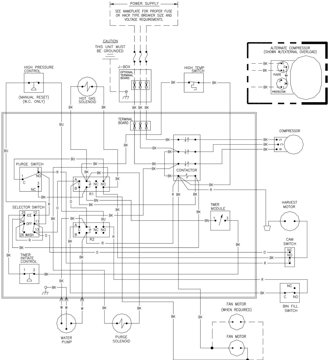
ICE1007 Air and Water Wiring Schematic
