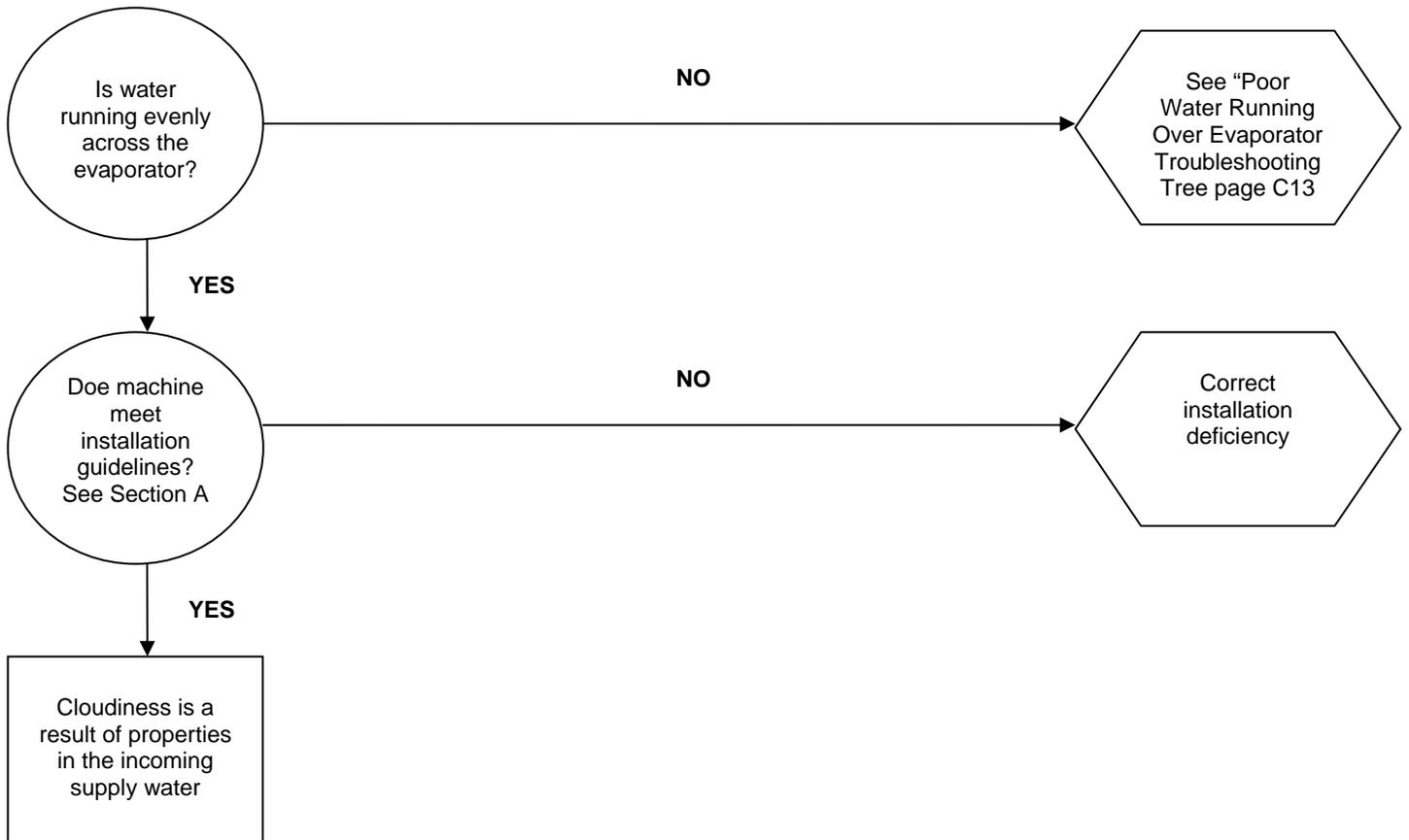
**Poor Water Distribution Over The Evaporator**
