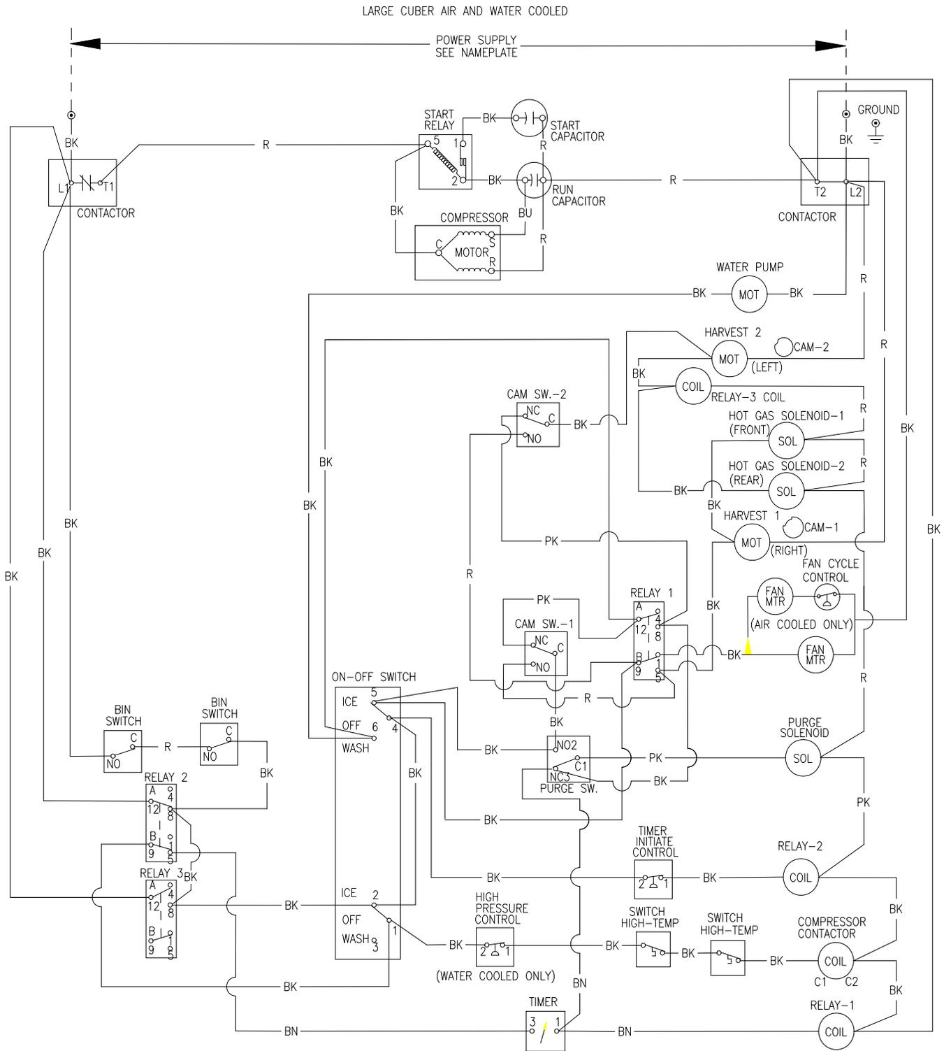
ICE1405/6A3/W3, ICE1806W3 and ICE2106W3 Wiring Schematic
