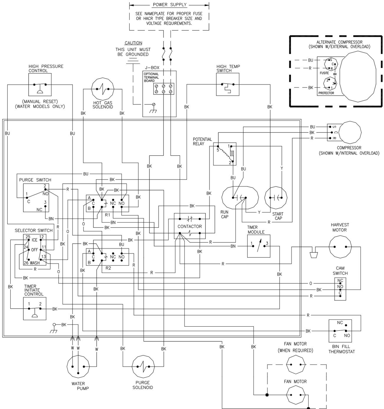
ICE0605/0606/0805/0806/1005/1006 Air and Water Wiring Schematic
