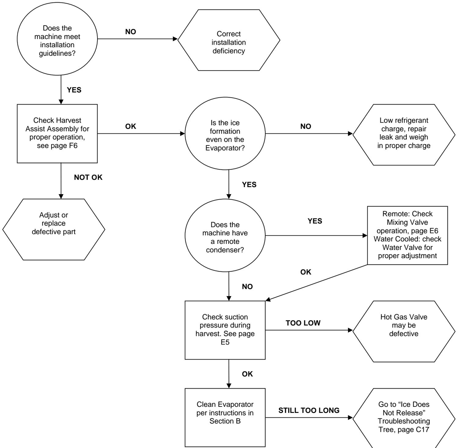
**Ice Does Not Release From Evaporator**
