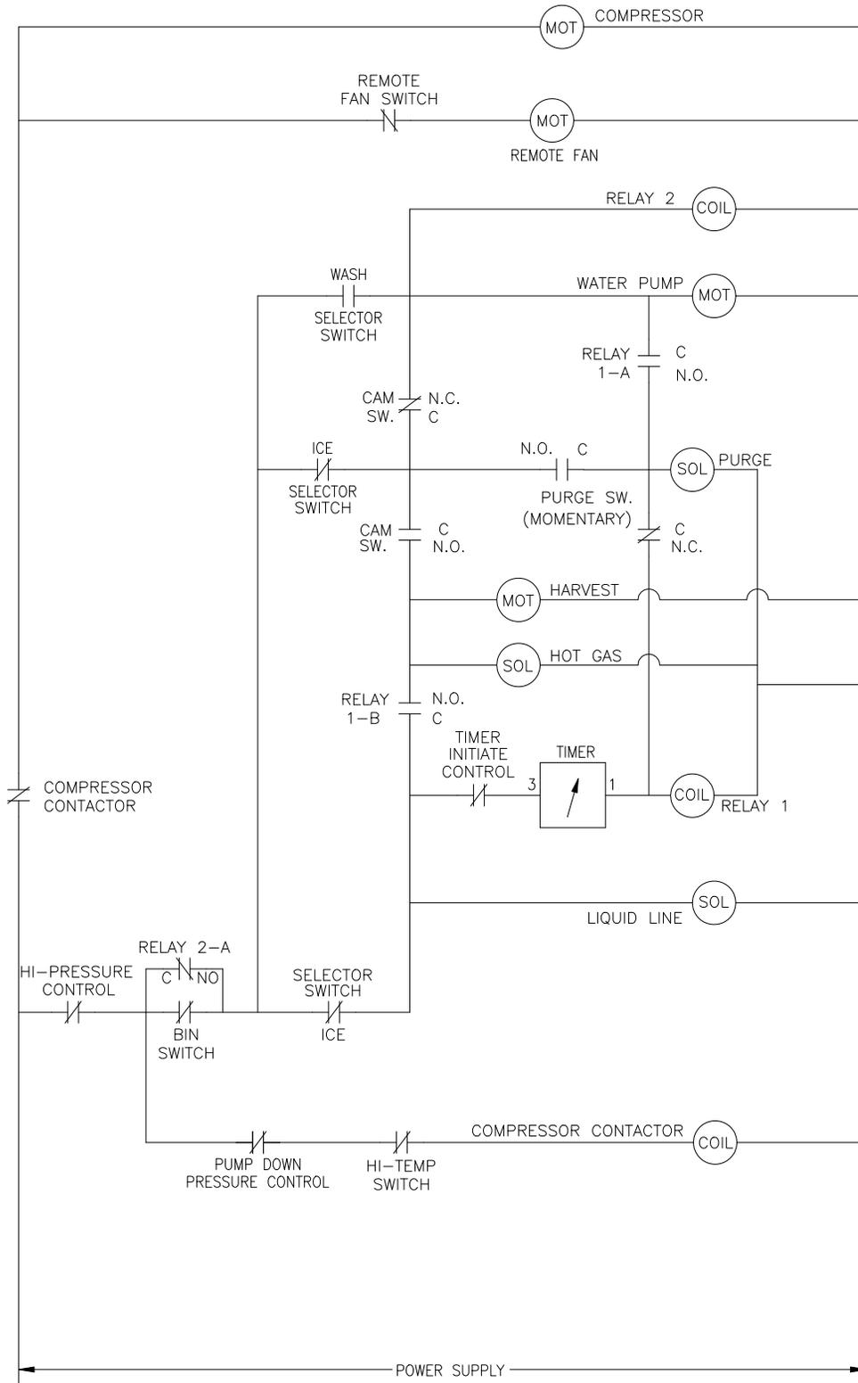
ICE1007 Remote Wiring Schematic (R3)
