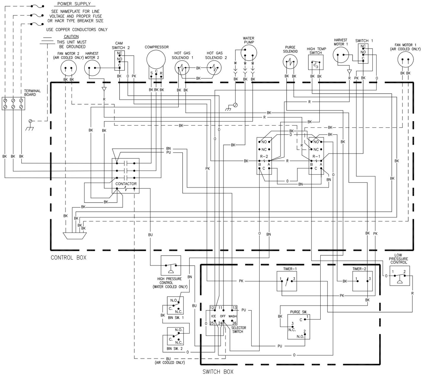
ICE1407/1807/2107 Remote Wiring Diagram
