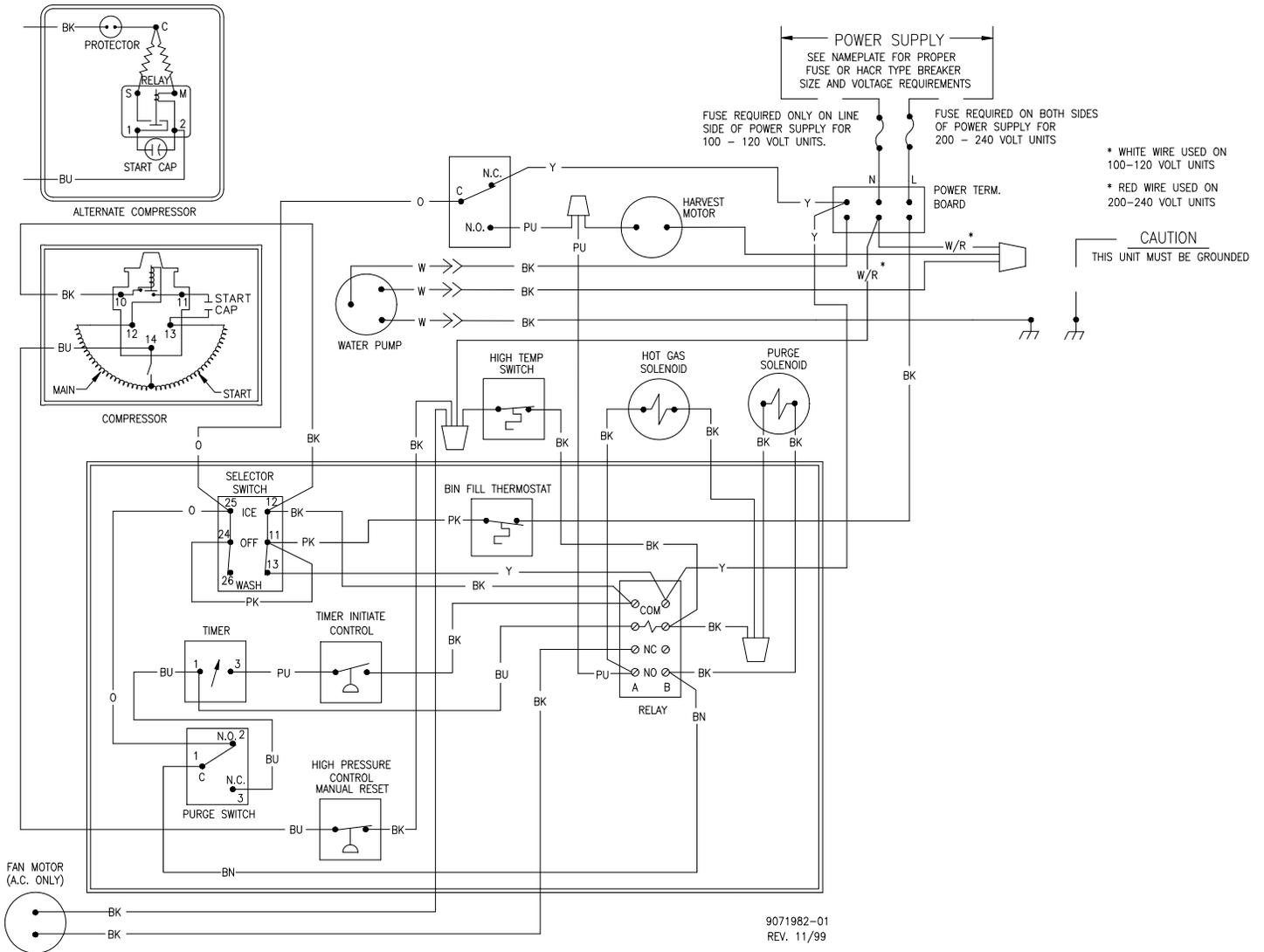
ICEU150/200/205/206 Air and Water Wiring Schematic
