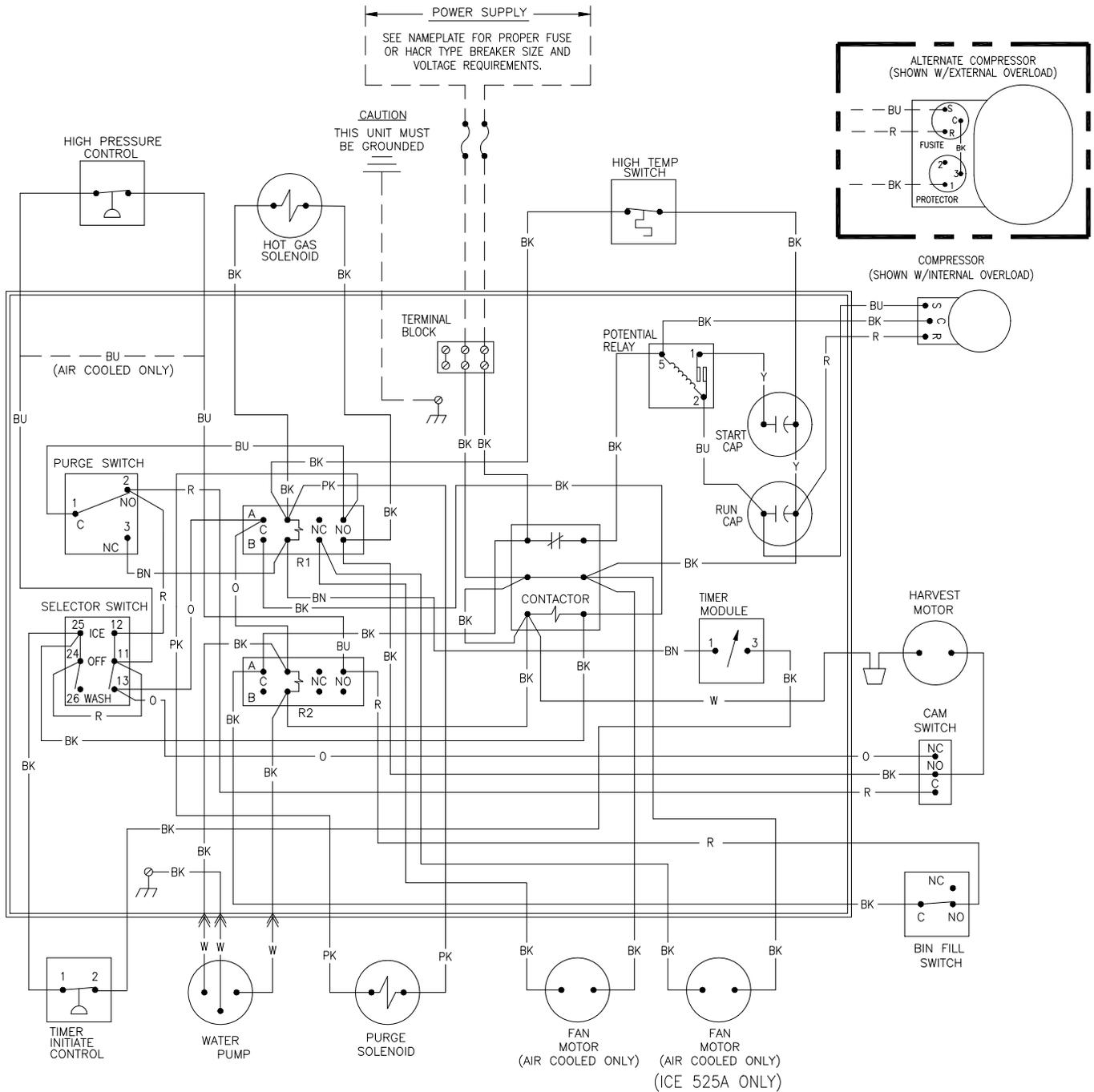
ICE0325/0525 Air and Water Wiring Schematic
