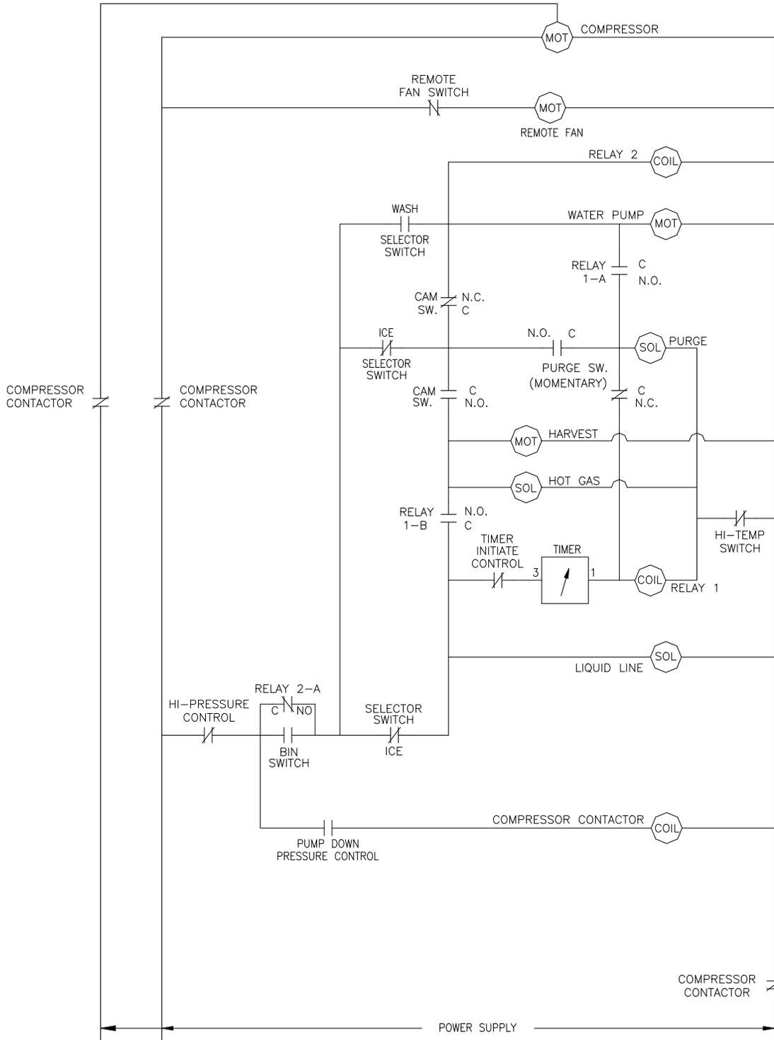
ICE1405/1406/1806/2005/2106 Air and Water Wiring Diagram
