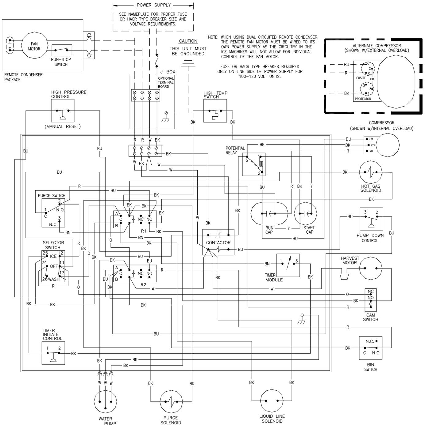
ICE0500 Remote Wiring Schematic
