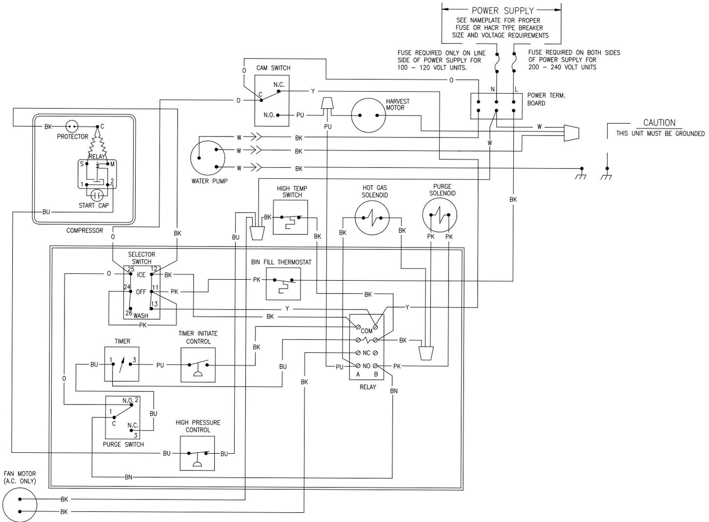
ICEU150/220/225/226 Air and Water Wiring Schematic
