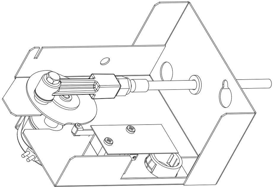
It takes approximately 1 minute for hot gas to heat the evaporator enough to loosen the ice from the evaporator plate. At this point the clutch pressure overcomes the capillary attraction of the ice to the evaporator plate and the ice begins to move off of the evaporator. As the ice is being pushed, the clutch stops slipping and begins to turn, extending the probe enough to push the ice completely off of the evaporator.
