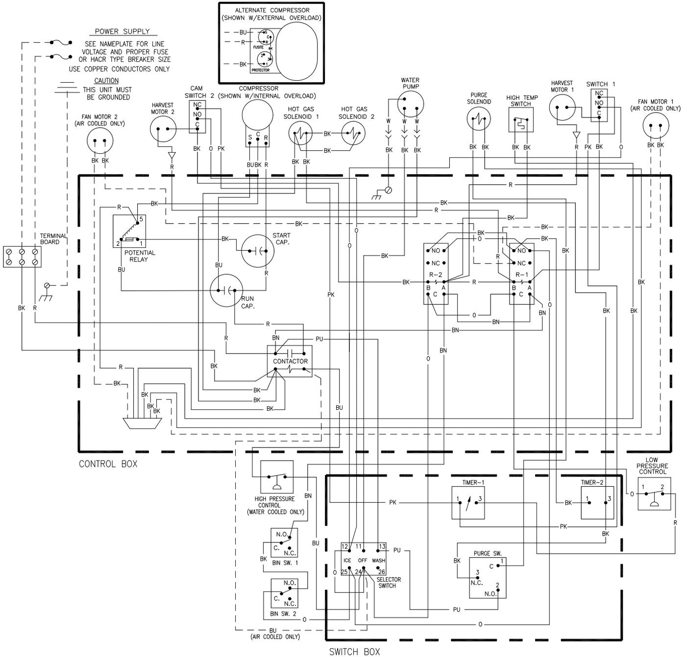
ICE1405/1406/1806/2005/2106 Air and Water Wiring Schematic
