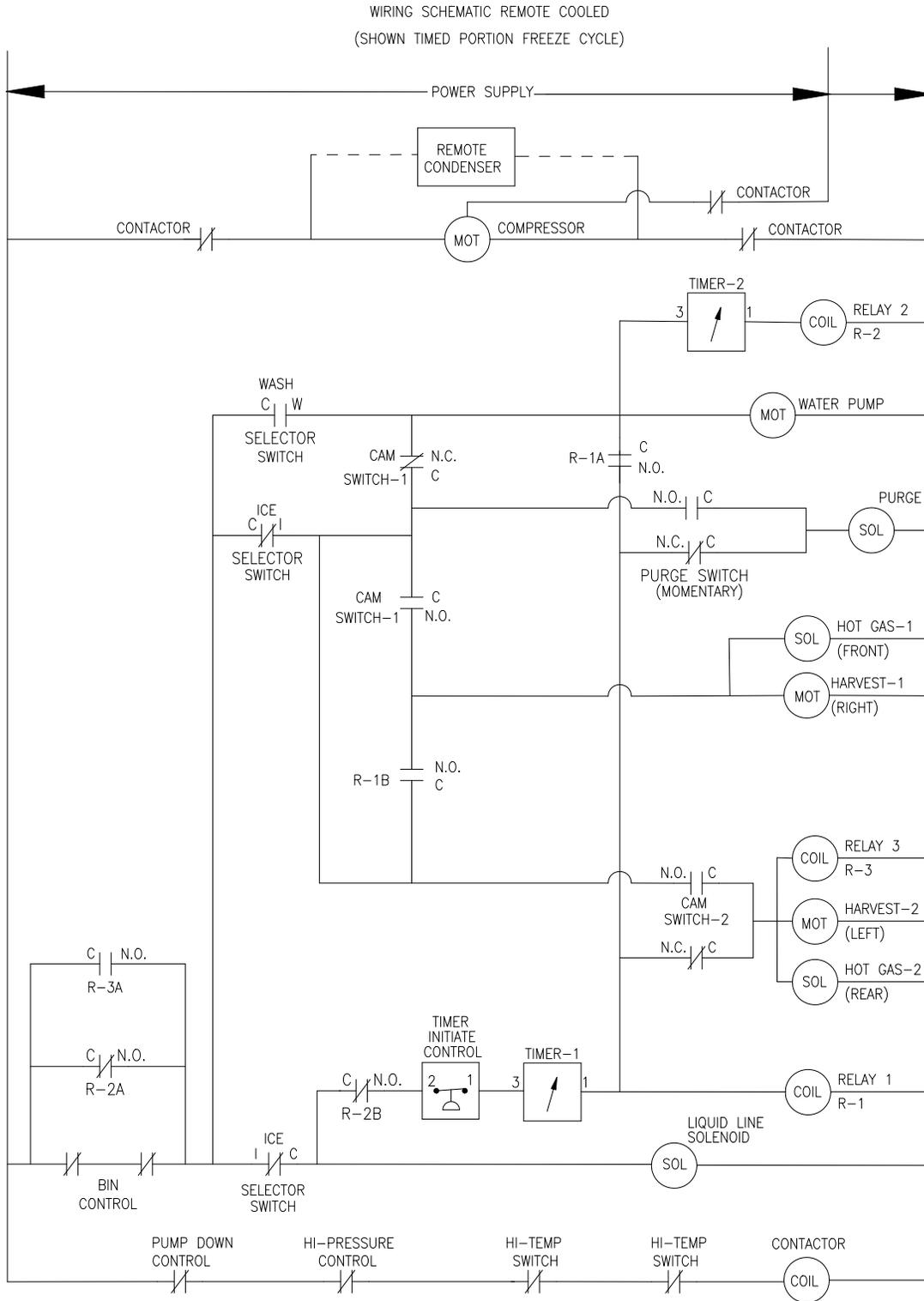
ICE1506R3 Wiring Diagram From Serial Number 09041280010750
