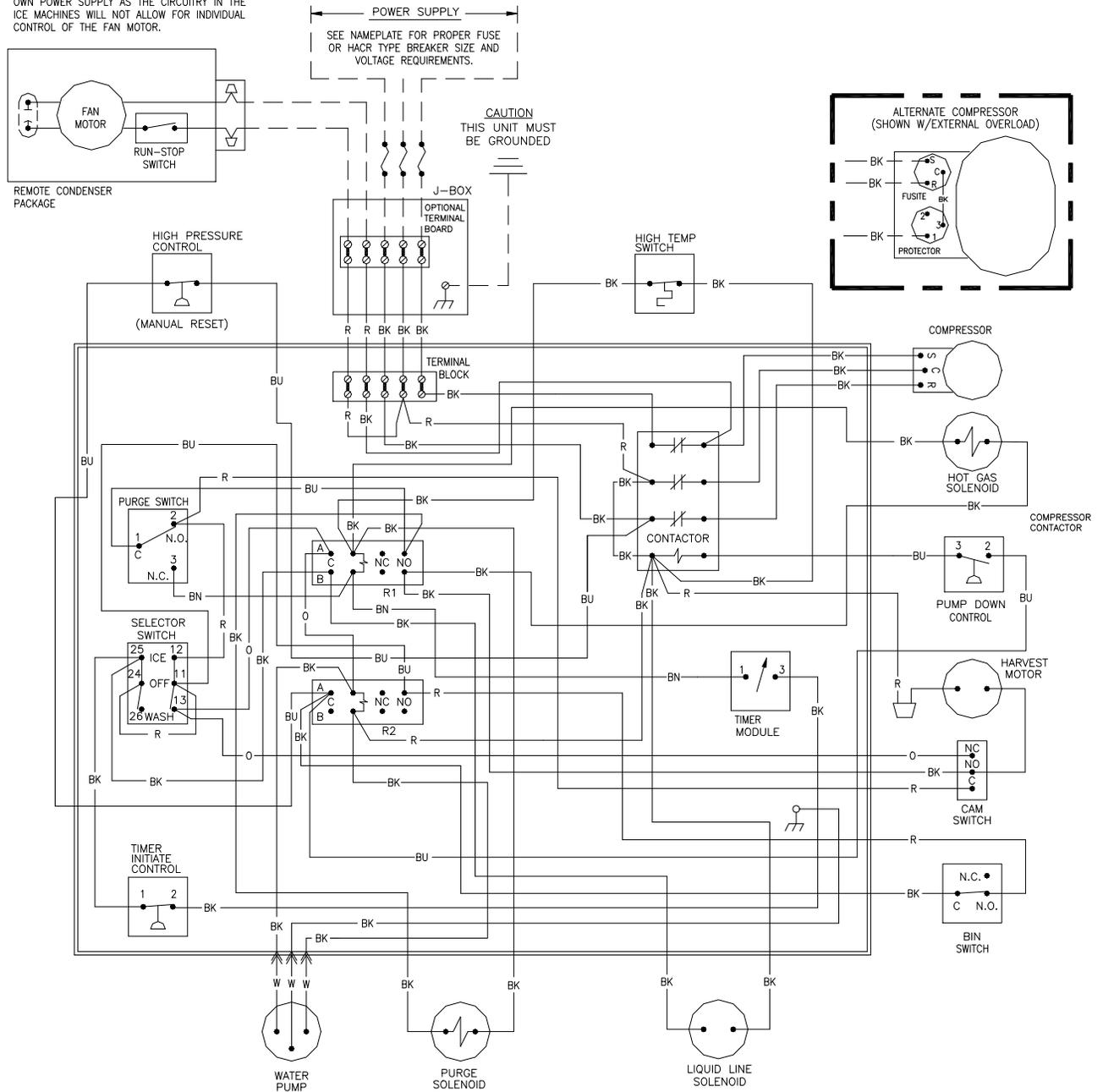
ICE1007 Remote Wiring Schematic
