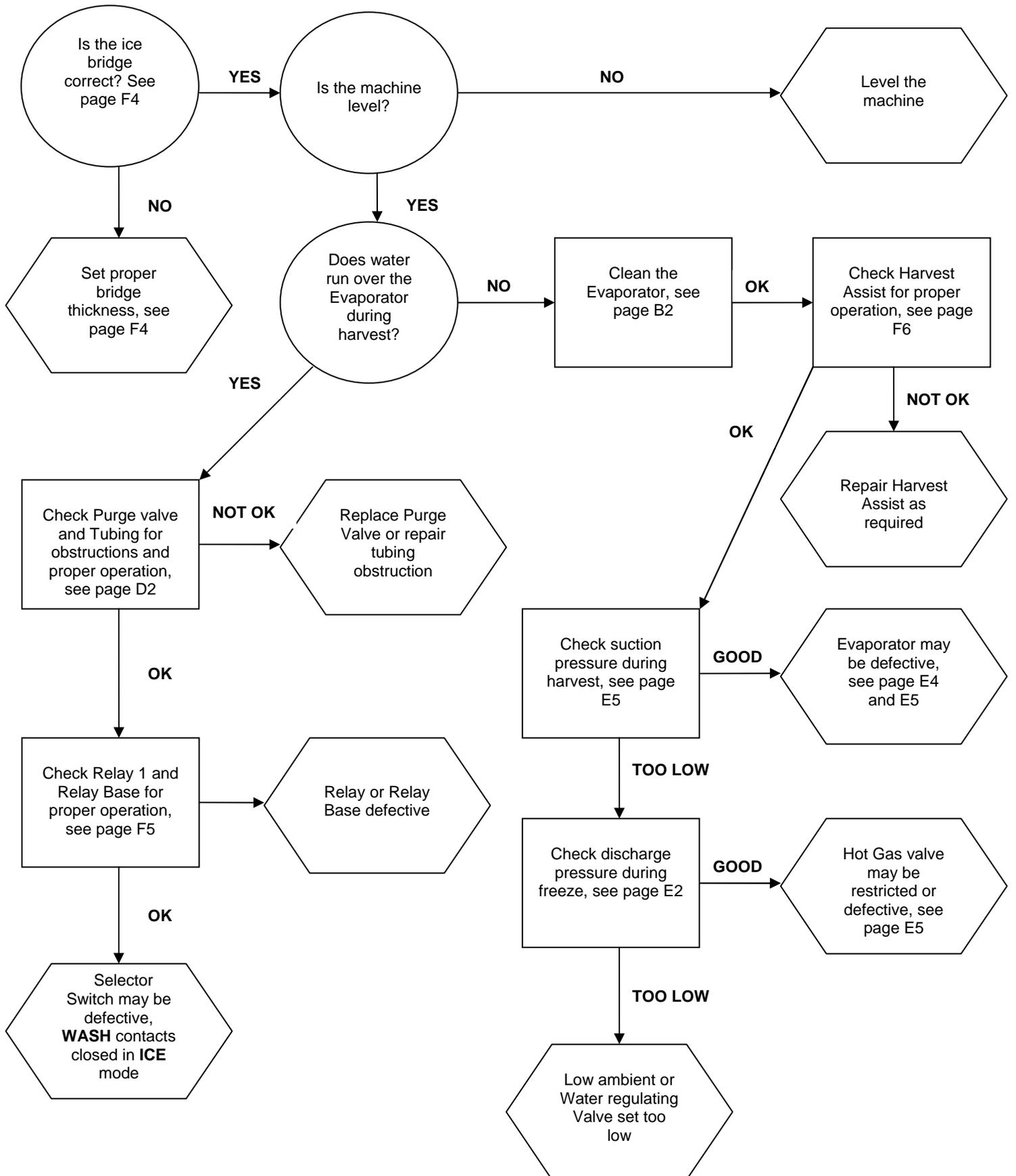
**Hot Evaporator, Low Suction And Discharge Pressure (Remote Only)**
