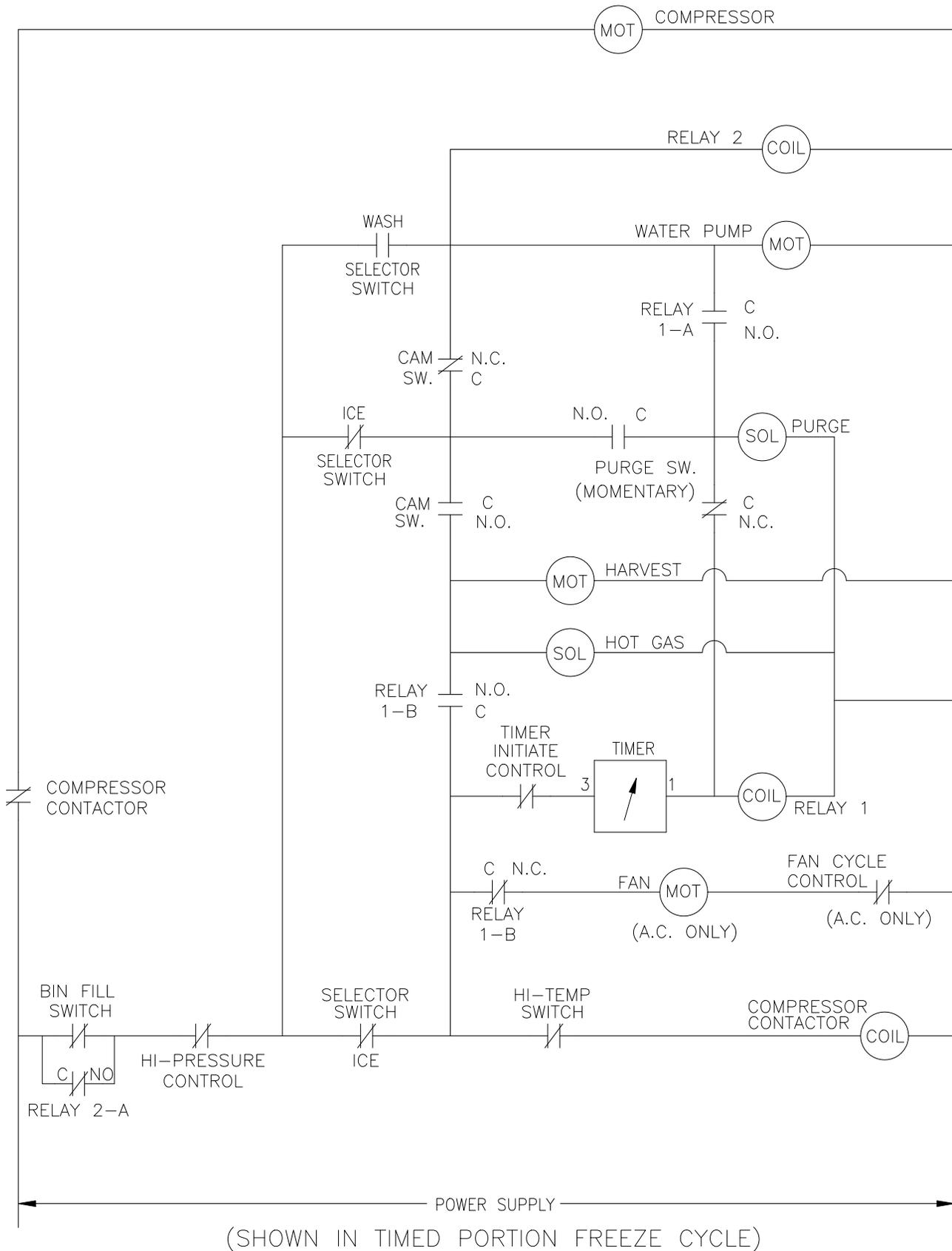
ICE0500 Remote4 Wiring Schematic
