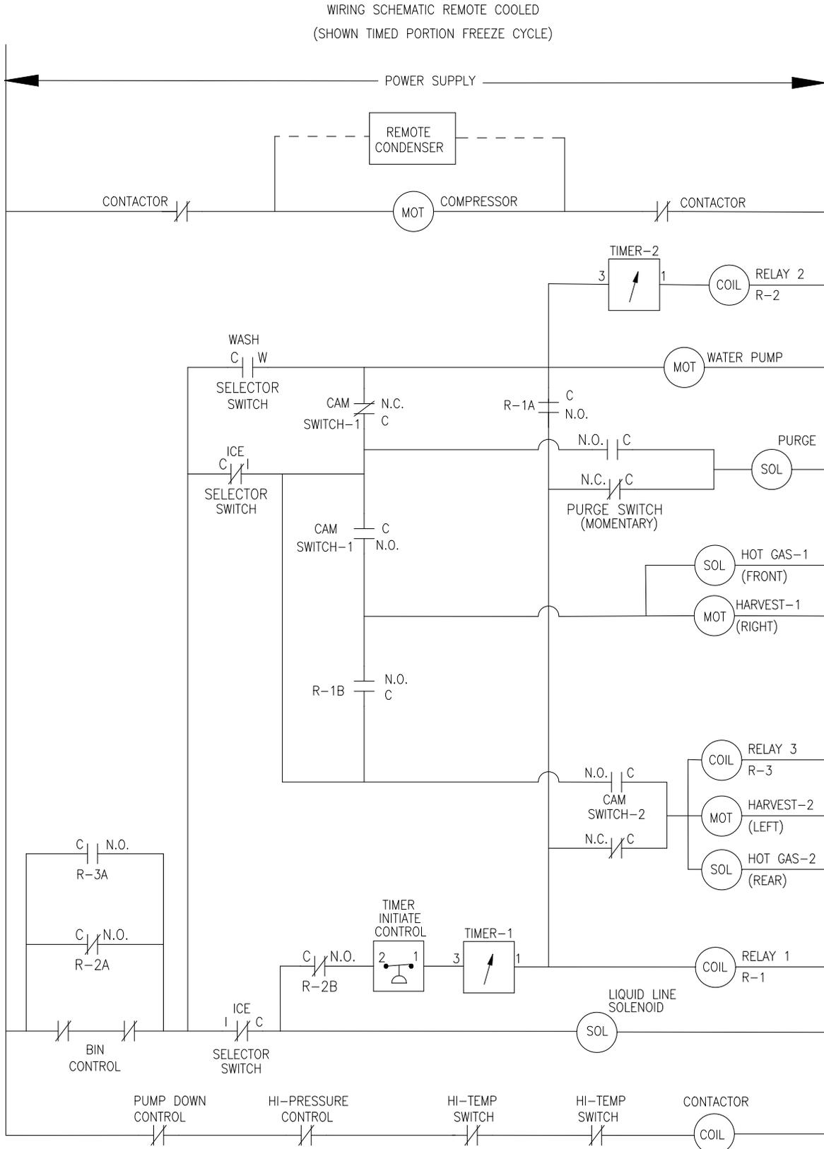
ICE1407R, ICE1807R, ICE2107R Wiring Diagram, From Serial Number 09041280010342
