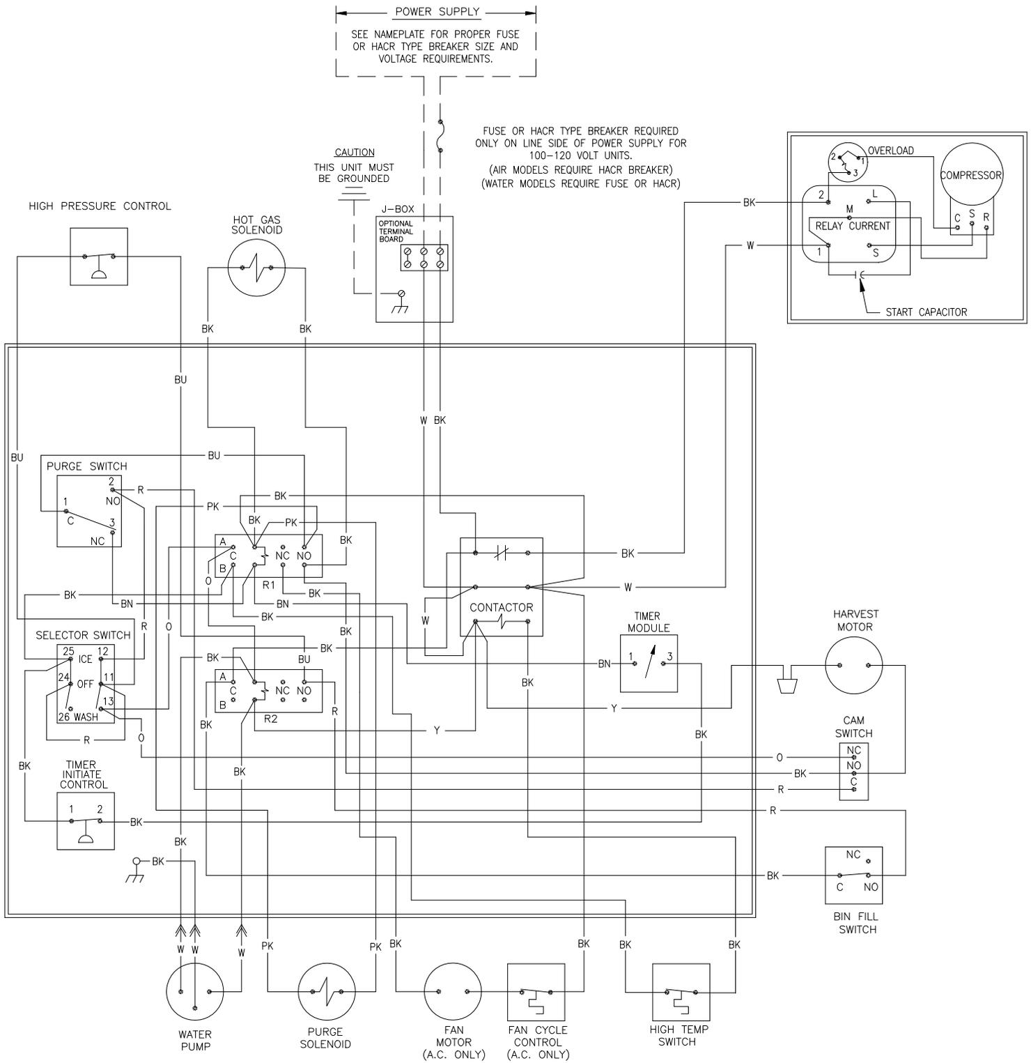
ICE0250 Air4 and Water4, ICE0400 Air3 and Water3 Wiring Schematic
