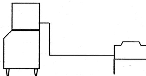
**DO NOT** Install any part of the refrigerant lines below the quick connect fittings at rear of machine.
