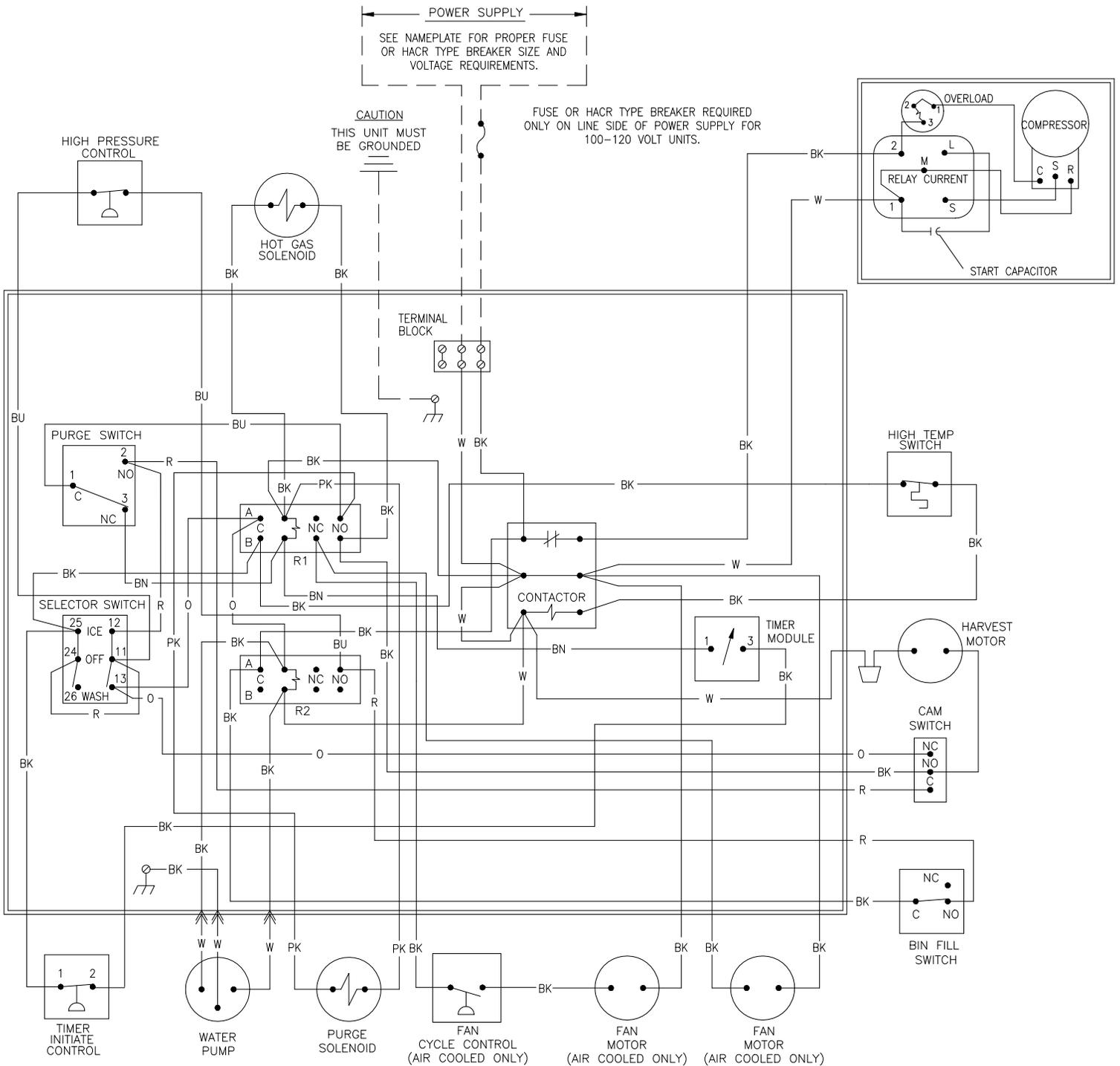
ICE0320 Air4 and Water4, ICE0520 Air3 and Water3 Wiring Schematic
