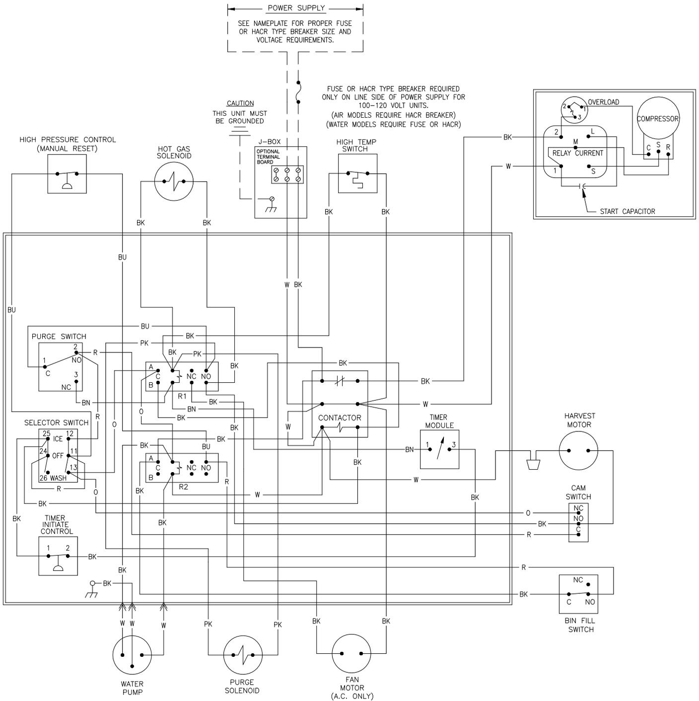
ICE0250 Air and Water Wiring Schematic
