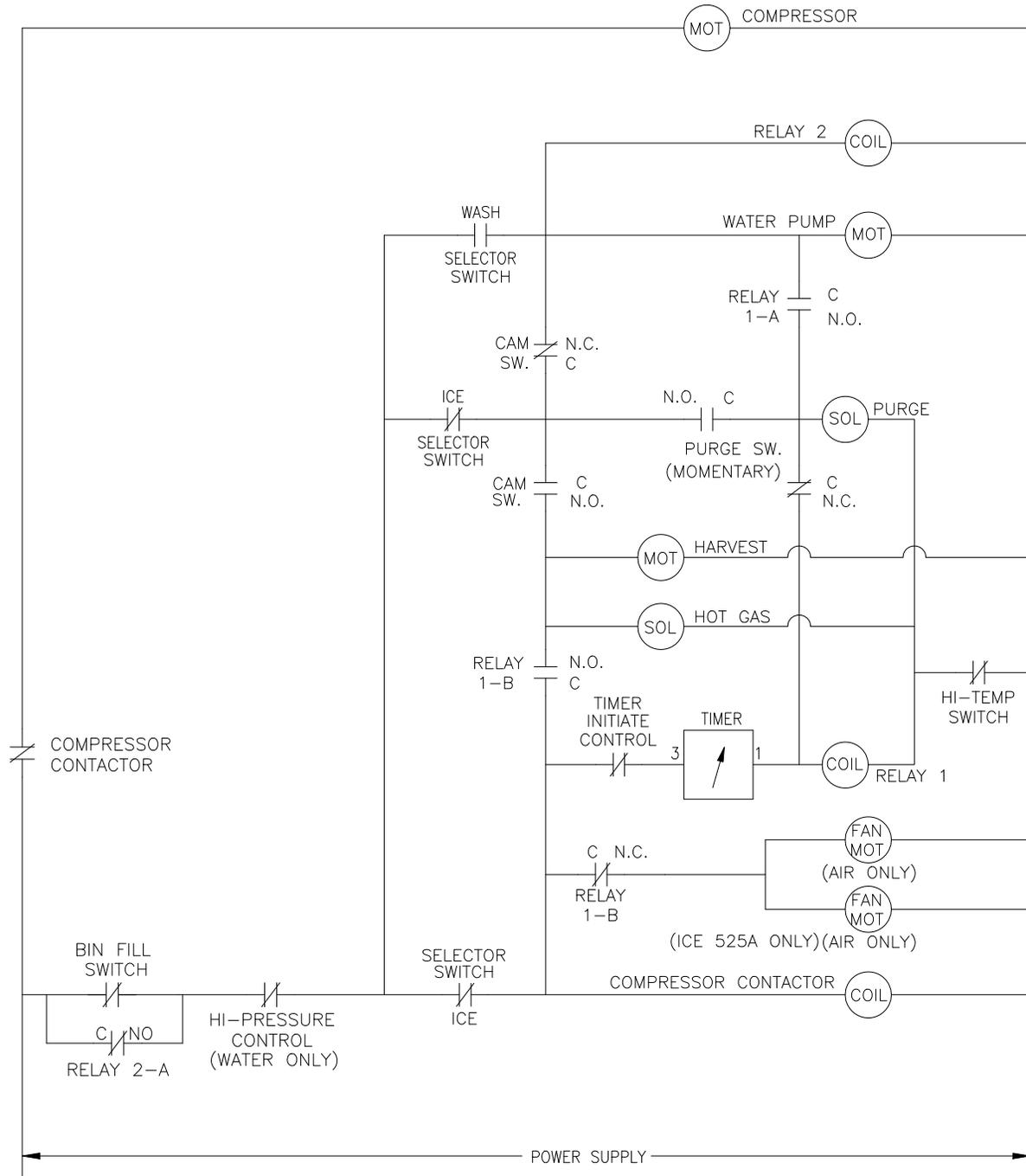
ICE0305 Air and Water Wiring Diagram
