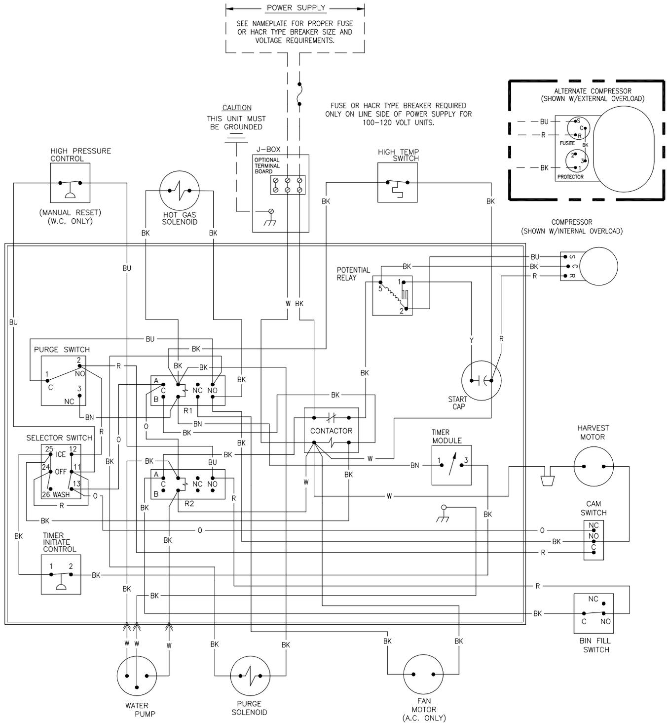
ICE0400 Air and Water Wiring Schematic
