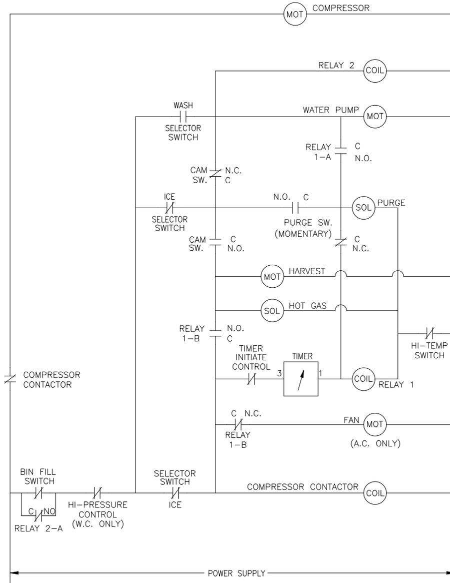
ICE0500 Air and Water Wiring Diagram
