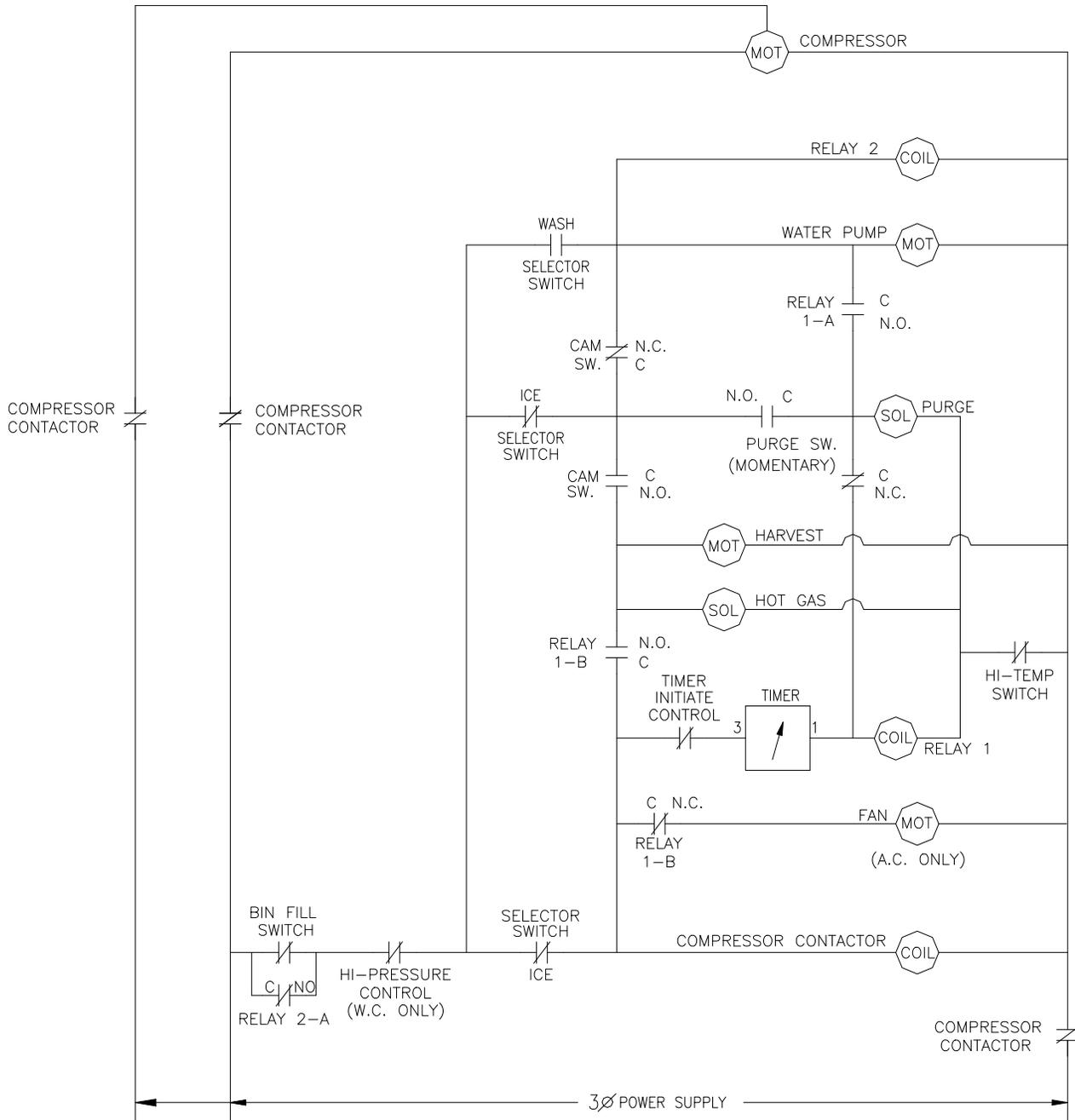
ICE1007 Remote Wiring Diagram
