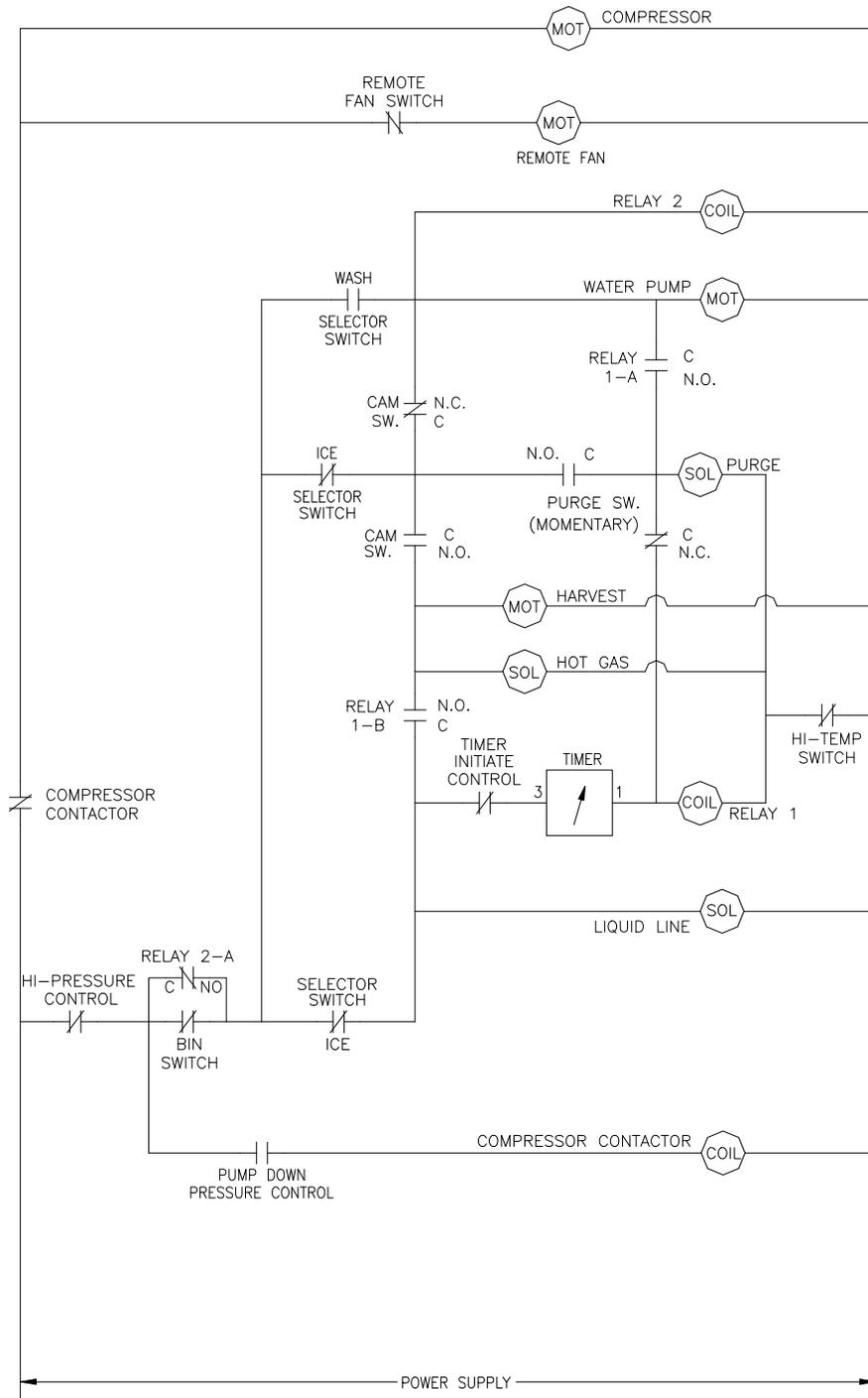
ICE1007 Air and Water Wiring Diagram
