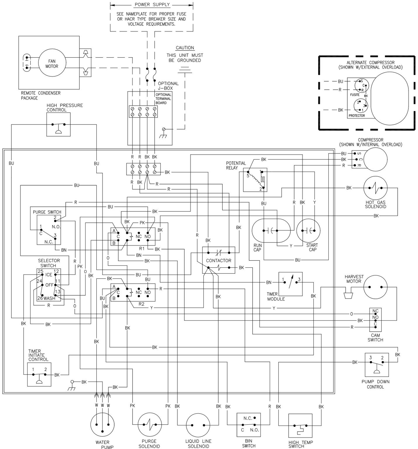
ICE0605/0606/0806/1006 Remote Wiring Schematic (R3)
