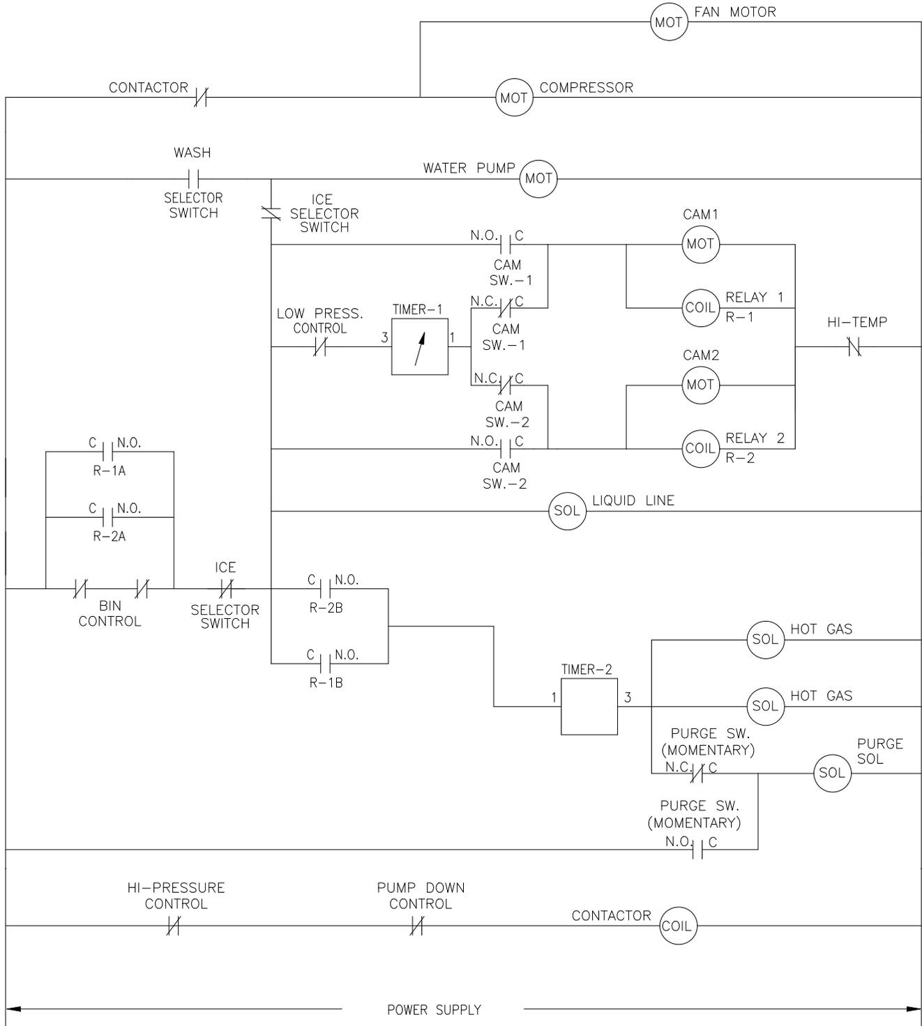
ICE0320 Air and Water Wiring Diagram
