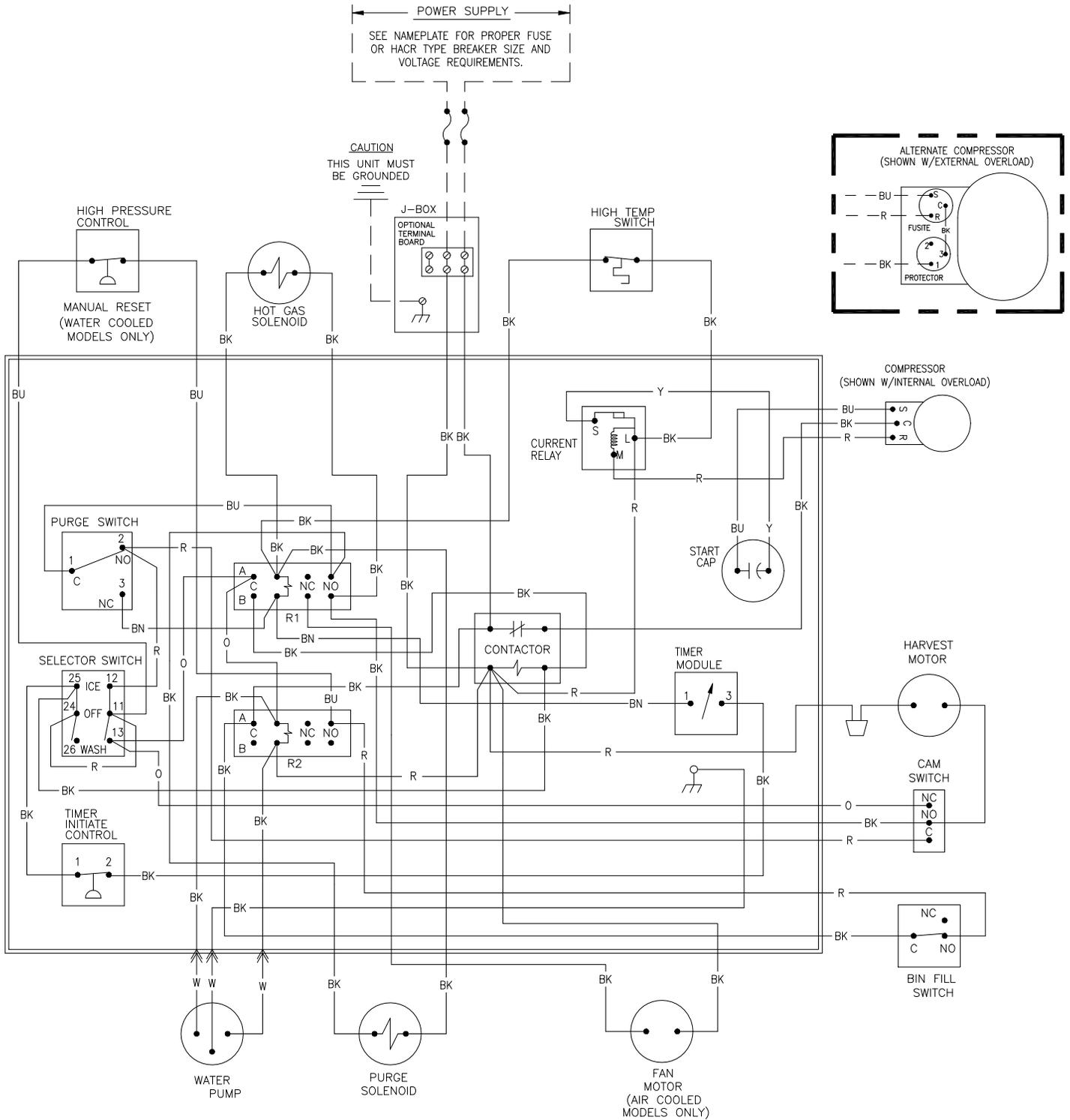
ICE0305 Air and Water Wiring Schematic
