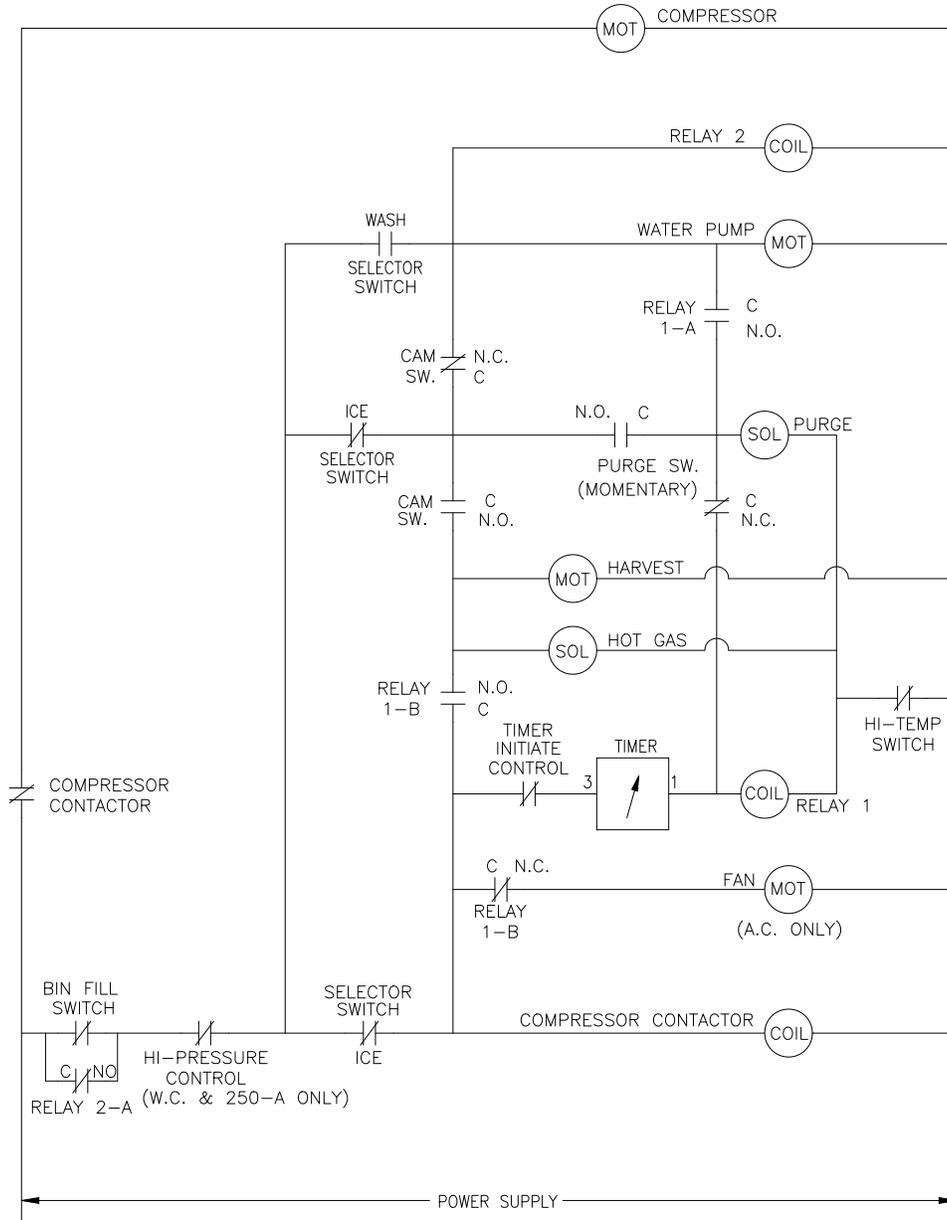
ICE0500 Remote Wiring Diagram
