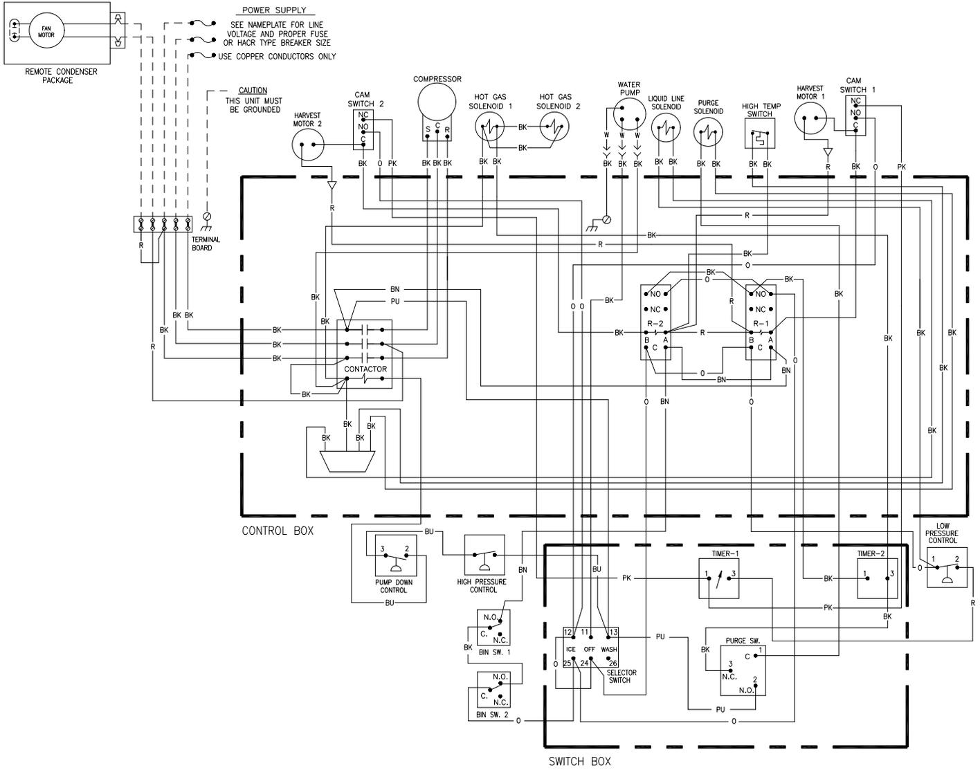
ICE1407/1807/2107 Remote Wiring Schematic
