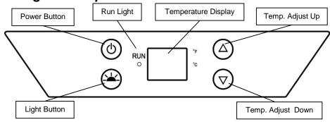
Use the up and down buttons to adjust the temperature. The temperature displayed can be in Fahrenheit or Celsius. This kegerator has a temperature range from 32°F to 60°F.
