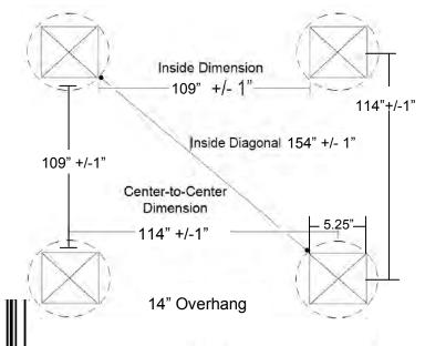
(Suggested for installation on lawns. For other surfaces, appropriate mounting methods should be used.)
