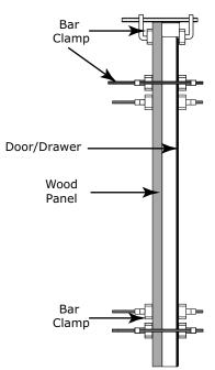
Using a 7/64" (3 mm) drill bit, drill 6 pilot holes into the wood panel 1/2" (12 mm) deep using the holes i
