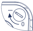
Fastener in locked position
