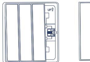
Note – For x14 'Press' retractive product, the switch will close contact when the rocker is removed. When fitting the rocker is recommended to turn on/off to ensure the contacts open.
