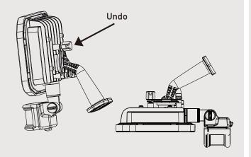
Fit floodlight to the wall using suitable fixings. Tilt and rotate floodlight to desired angle and securing fixing bolt. Ensure product is secure.
