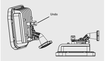
Fit floodlight to the wall using suitable fixings. Tilt and rotate floodlight to desired angle and securing fixing bolt. Ensure product is secure.
