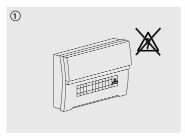
Turn OFF power supply, ensure all required equipment and tools are present. For optimal detection, avioid placing near sources of heat e.g. extractor vents
