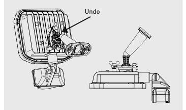
Fit floodlight to the wall using suitable fixings.
