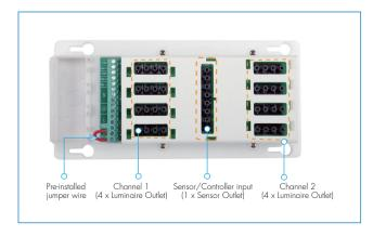
By removing this pre-installed jumper wire, the 8 outlets are then divided into two separate channels. This LPCHTKQCB1-01 becomes a 2-channel box with 2 x 4 luminaire outlet. The two channels will be controlled separately (Channel 1 is controlled by Switched L1, and Channel 2 is controlled by Switched L2).
