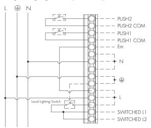
Note: 1. A local lighting switch may still be used when there is a central emergency test switch or when a circuit breaker is used to interrupt the power.
