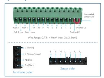
Factory default for LPCHTKQCB1-01 comes with a pre-installed jumper wire, which short-connects Switched L1 and Switched L2 together. With this jumper wire, all the 8 luminaire outlet are considered as in a same channel (1  $\times$  8) that are controlled together by the sensor/controller.
