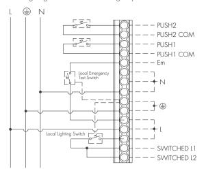
Using Local lighting switch for power interruption
