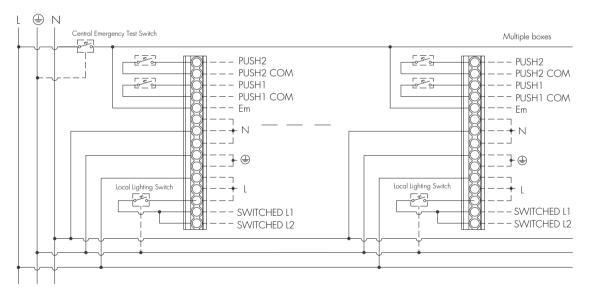
Note: 1. A local lighting switch may still be used when there is a central emergency test switch.
