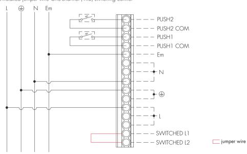
Note: 1. For two-channel (2x4) switching control please remove the jumper wire.
