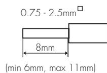
Pluggable screw terminal. It is recommended to make connections to the terminal before fitting to the sensor.
