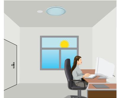
The sensor switches off the light when natural light is sufficient, even with presence.
