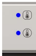
Fig. 12 Indicator light for chamber and boiler heaters
