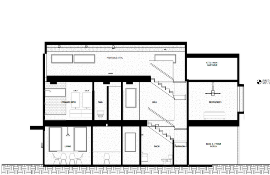
1 BLDG 1 - SECTION 1 SCALE: 1/4" = 1'-0"
