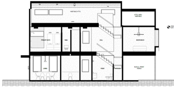
1 BLDG 1 - SECTION 1 SCALE: 1/4" = 1'-0"
