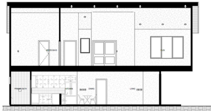
2 BLDG 1 - SECTION 2 SCALE 1/4" = 1'-0"
