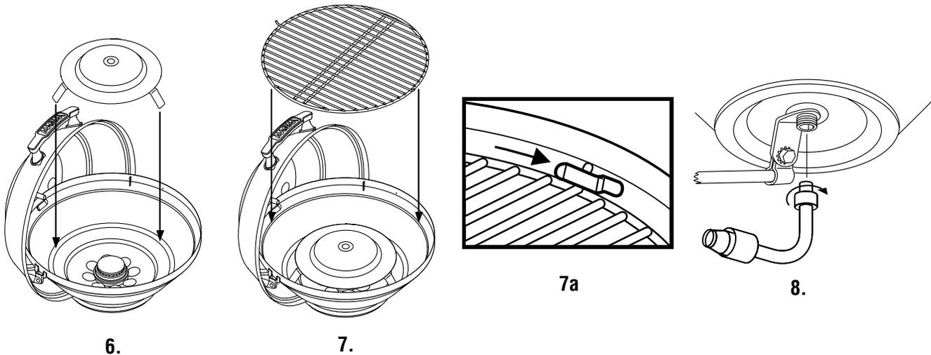
6. Install radiant plate over burner on bowl ridge.
