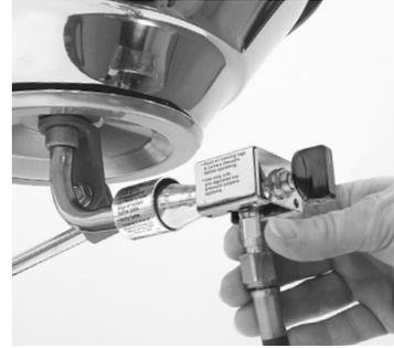
Gently insert valve stem into venturi tube upside down until fully inserted and rotate as shown.
