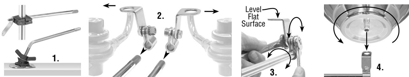
1. Select and install appropriate Magma mount in your desired location. Prior to installing the grill, check that mount does not easily move with a reasonable force applied.
