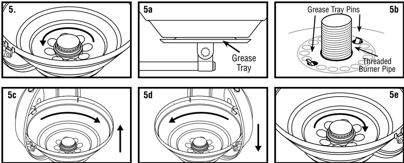
5. With grill body tightly attached to L-Bracket, unthread burner counter-clockwise **3 full revolutions only**. **CAUTION: DO NOT UNTHREAD MORE THEN 3 REVOLUTIONS, AS GRILL MAY FALL OVERBOARD.**
